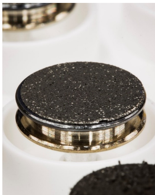
Figure 3.12: Example of sediment mounted to stub for SEM analysis (diameter = 12.5mm).
