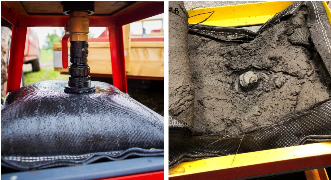
Figure 5.11: Geotextile bag following 200 L filtration trial (A), and immediately following dissection (B).
