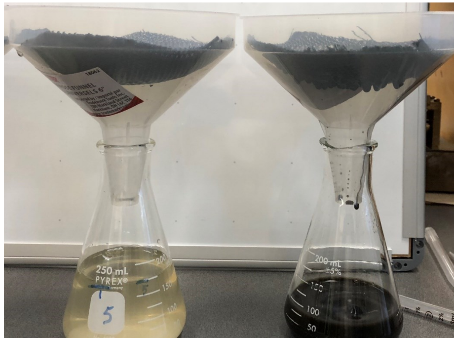
Figure 3.6: Bench scale dewatering trial of raw and treated slurry.
