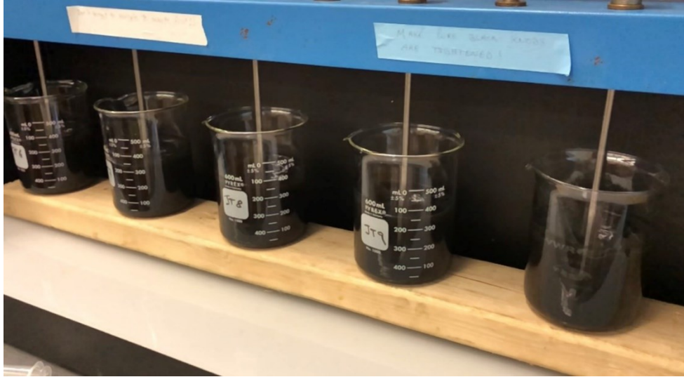
Figure 3.5: Jar test on 4 of 9 selected dosages (JT 6 – 9) and raw 1% slurry.
