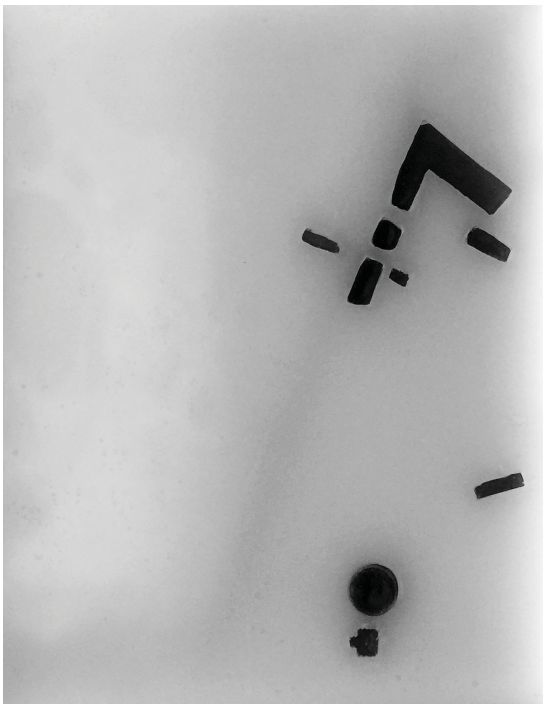
Material transparency test, two 8 mm layers of cast wax, building footprints in graphite-saturated wax for pigment, road in wood.
