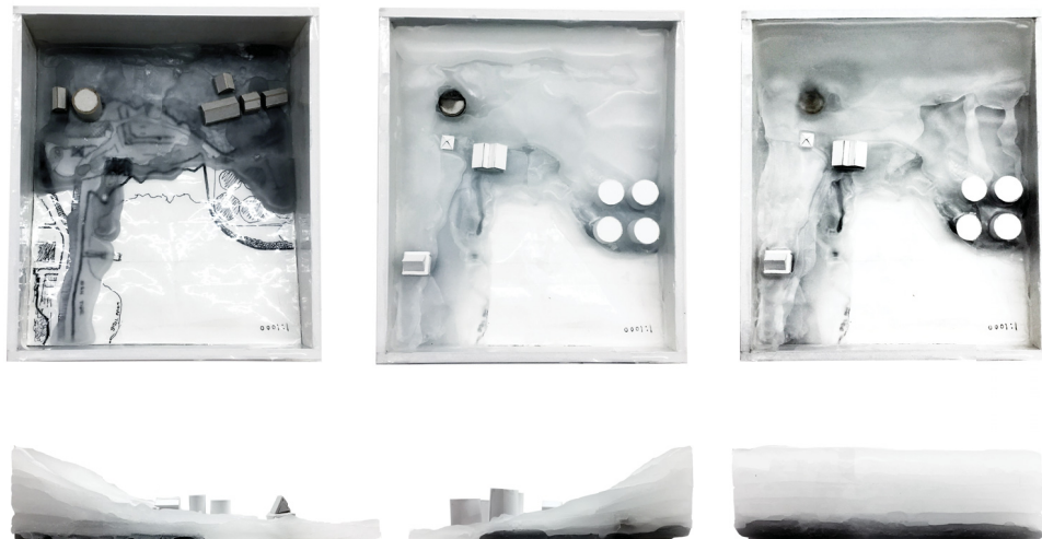
Layering process of poured wax to create solidified landscape sketch site model
