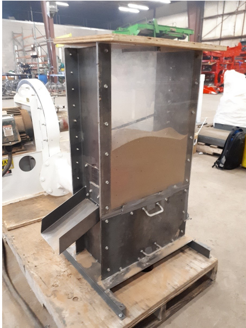
Figure 42.b) Photograph of the fluidized bed built
