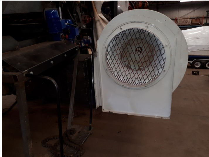
Figure 29. The fan moved from the top of the harvester and mounted at the inlet of the plenum
