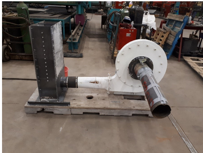
Figure 42 a) Photograph of the fan of the fluidized with inlet flow measurement duct
