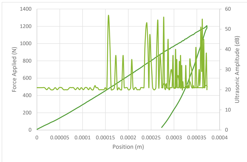
Figure 60: 2Ni-P micro indentation result
