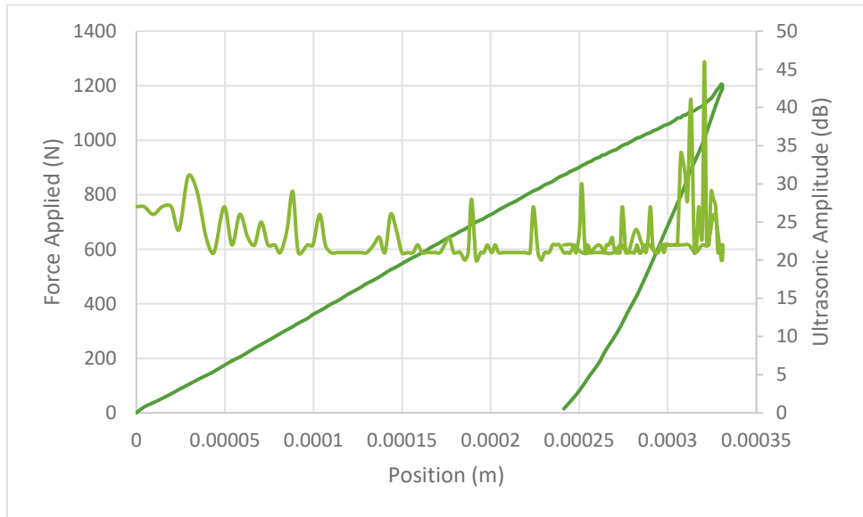
Figure 66: 2 hr Ni-P-W micro indentation result
