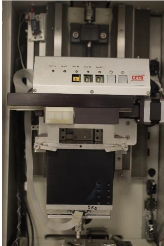
Figure 8: CETR scratch tester
