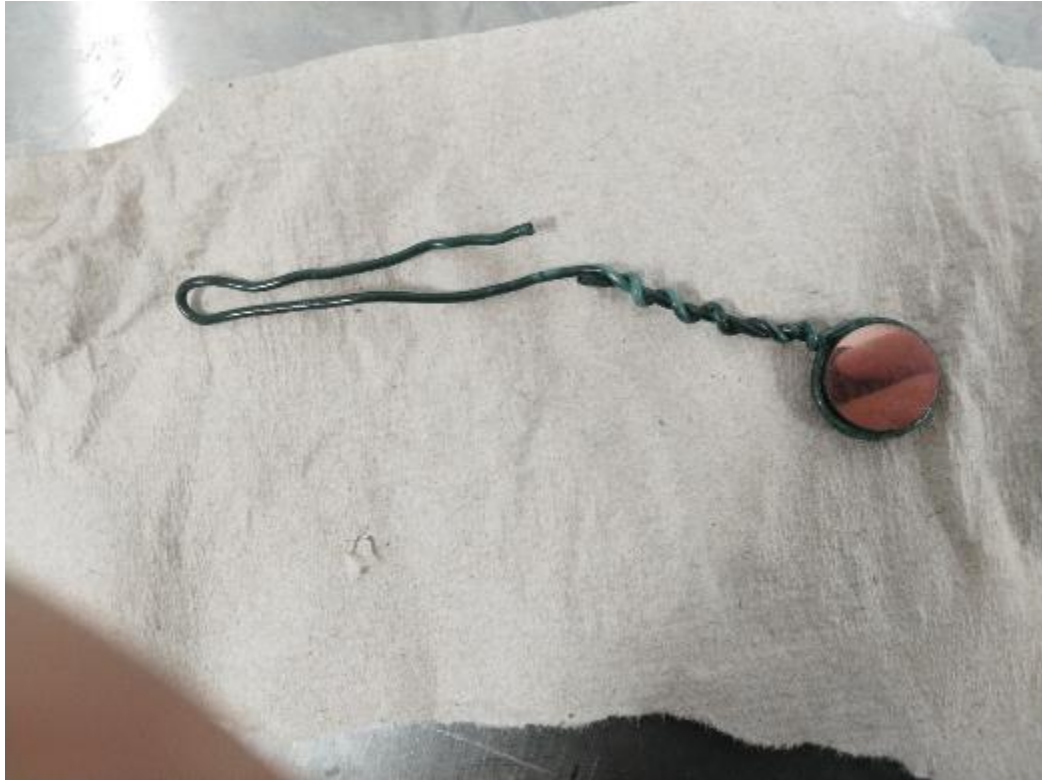
Figure 10: Electroless coating sample holder
