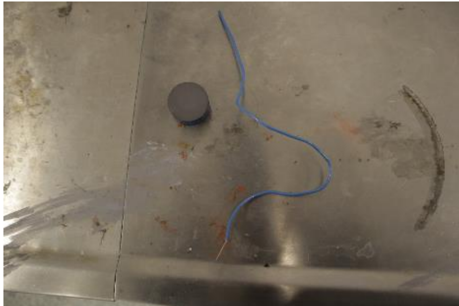
Figure 18: Broken wire from anode at connection point
