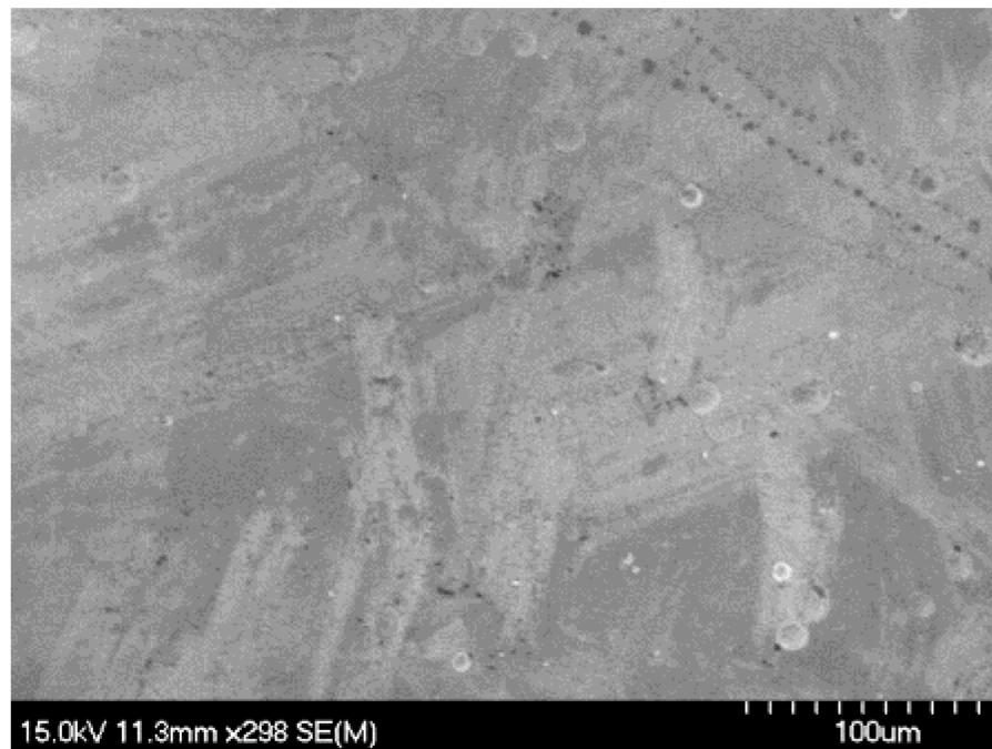
Figure 30: SEM of Electroless coating (Atotech solution, Ni-P, 95 °C, diamond polished, 2 h) (low magnification) (smooth surface)
