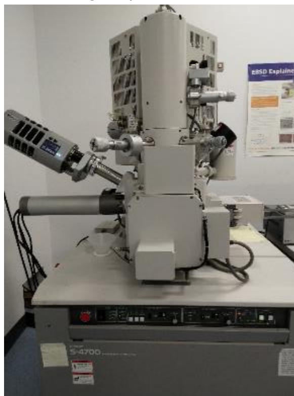
Figure 5: Hitachi S-4700 scanning electron microscope with vacuum pump below
