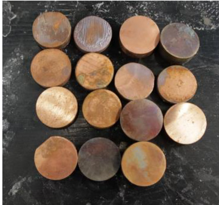
Figure 15: Samples failed to electroless plating with purple streaks
