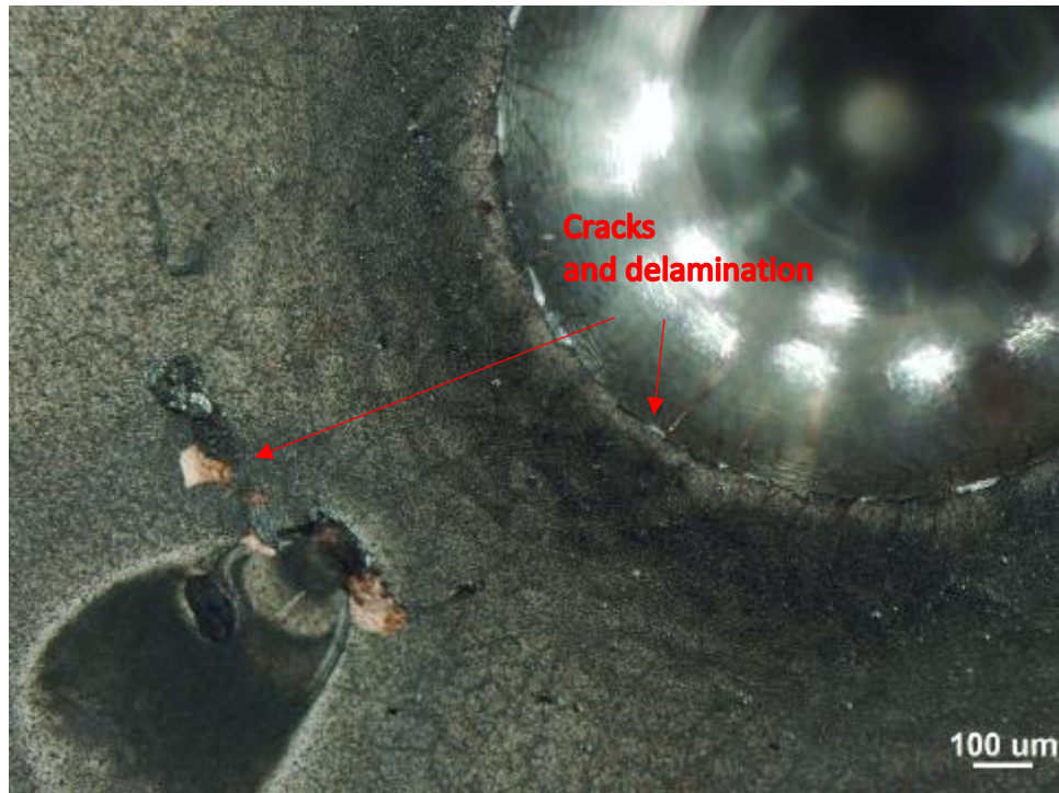
Figure 70: Micrograph of 3 hour Ni-P-W plating indentation result
