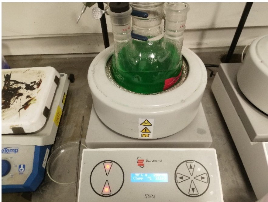
Figure 4: Electroless coating set up with Electrothermal heat mantle
