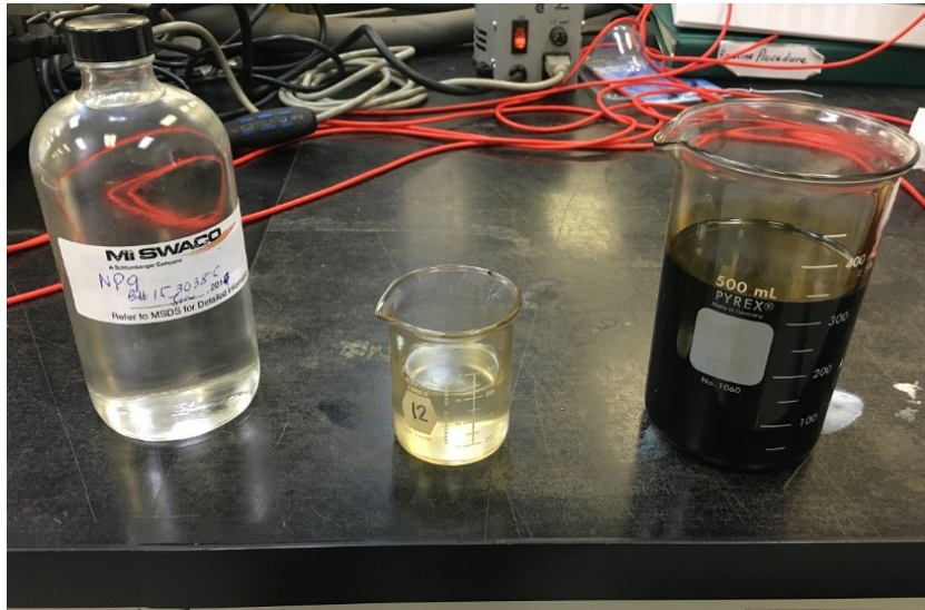
Figure 3-1: Illustration of the raw materials required to conduct the experiment. The raw materials are listed from left to right as follows; reservoir connate water, stabilizing agent and dead crude oil.
