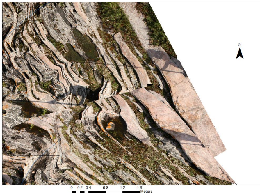
Figure 7.1: A close up of ArcMap showing a photofault in a region of change in elevation. It is clear to see, the panoramas do not overlap perfectly.
