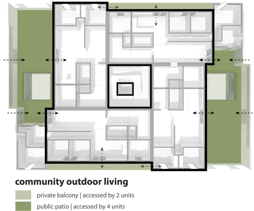
Figure 50: Each unit has access to a private balcony (two units per) and a public patio (four units per).
