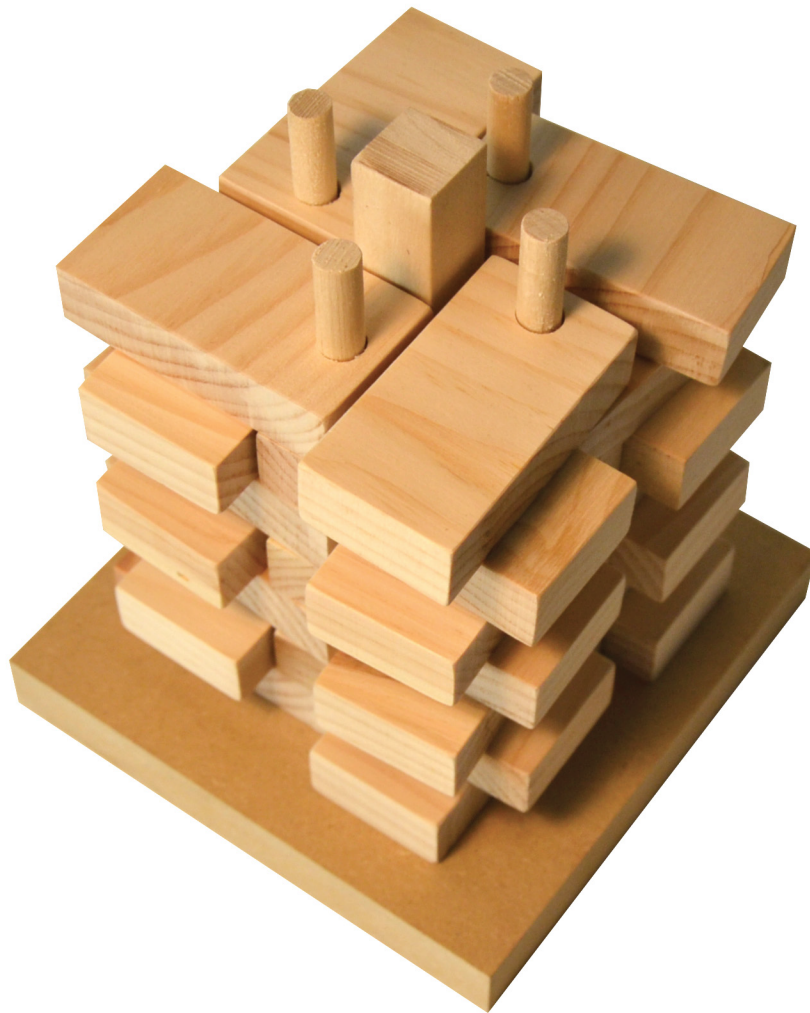
Figure 47: The building model demonstrates the rotated module around the circulation core, with continuous vertical plumbing cores anchoring the units. Each floor is a mirrored plan of the floor above/below.
