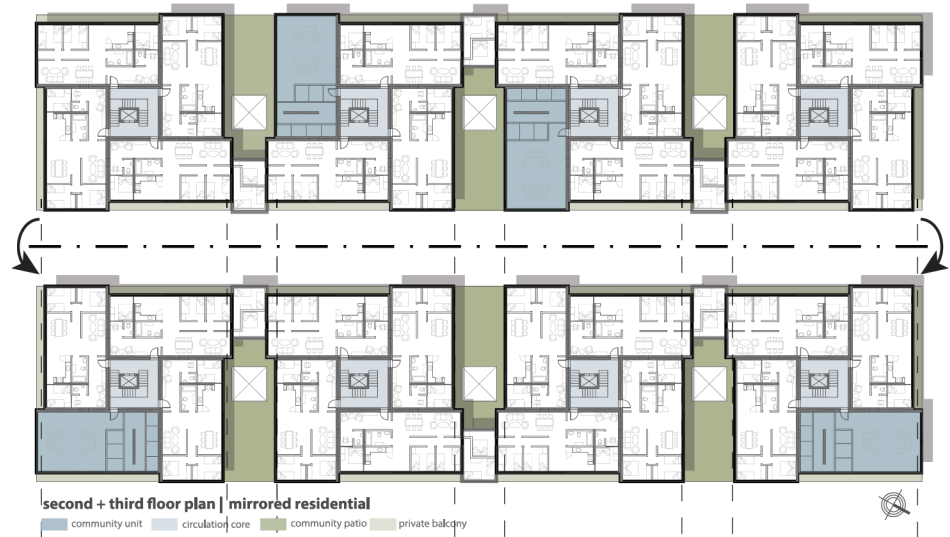
Figure 49: Floor plans are composed of four unit clusters (four units rotate around one circulation core, per cluster) that are connected by an exterior public patio. Alternating floors are mirrored plans, while retaining continuous plumbing and circulation cores.
