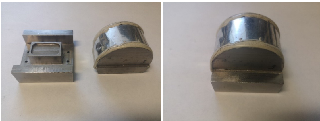
Figure 2.3 Air sensitive XRD holder before (left) and after (after) assembly.
