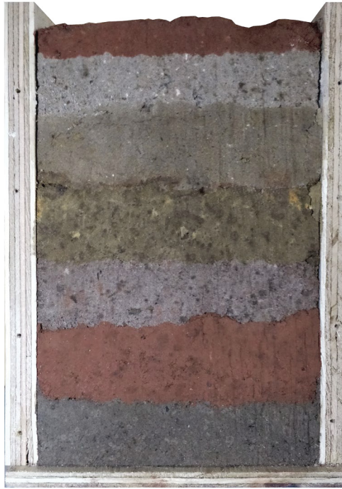
Figure 46 is a photograph of the outcome of the rammed earth experiment.
