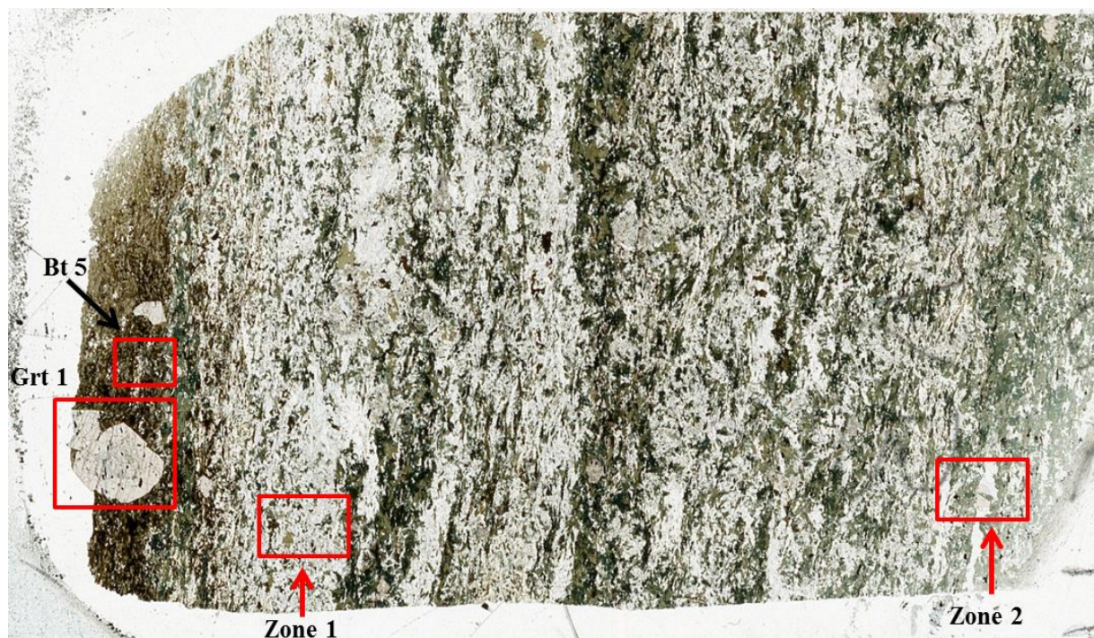
Figure 3.6: Scanned polished section of Int1-B showing the zones where analyses were conducted. Back-scattered electron images of the zones are shown in Figure 3.7 (Grt 1), Figure 3.8 (Zone 1), and Figure 3.9 (Bt 5). Analyses from Zone 2 were not used in P-T calculations. Note that the term “zone” as applied here refers to an area where points of analysis were selected and not to specific textural and/or mineralogical domains.
