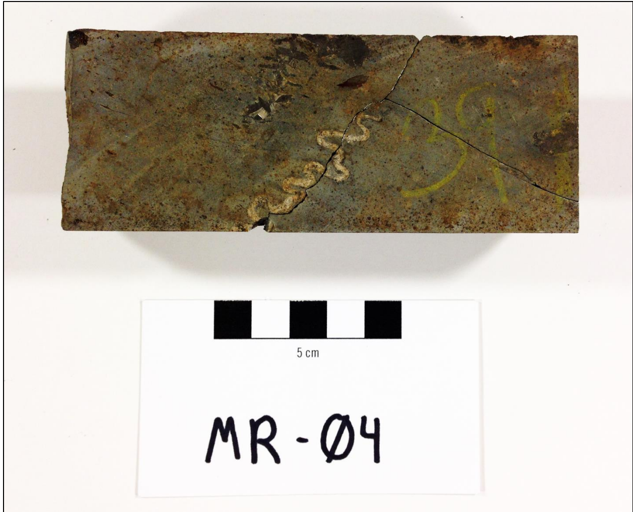
Figure 4.3: Core sample MR-04. The photo was taken while the core was dry. Note the large arsenopyrite crystals in the middle of the top edge; gold is visible within those crystals under the electron microprobe. The serpentine veinlet of carbonate indicates buckling representing ~45% shortening perpendicular to incipient foliation.
