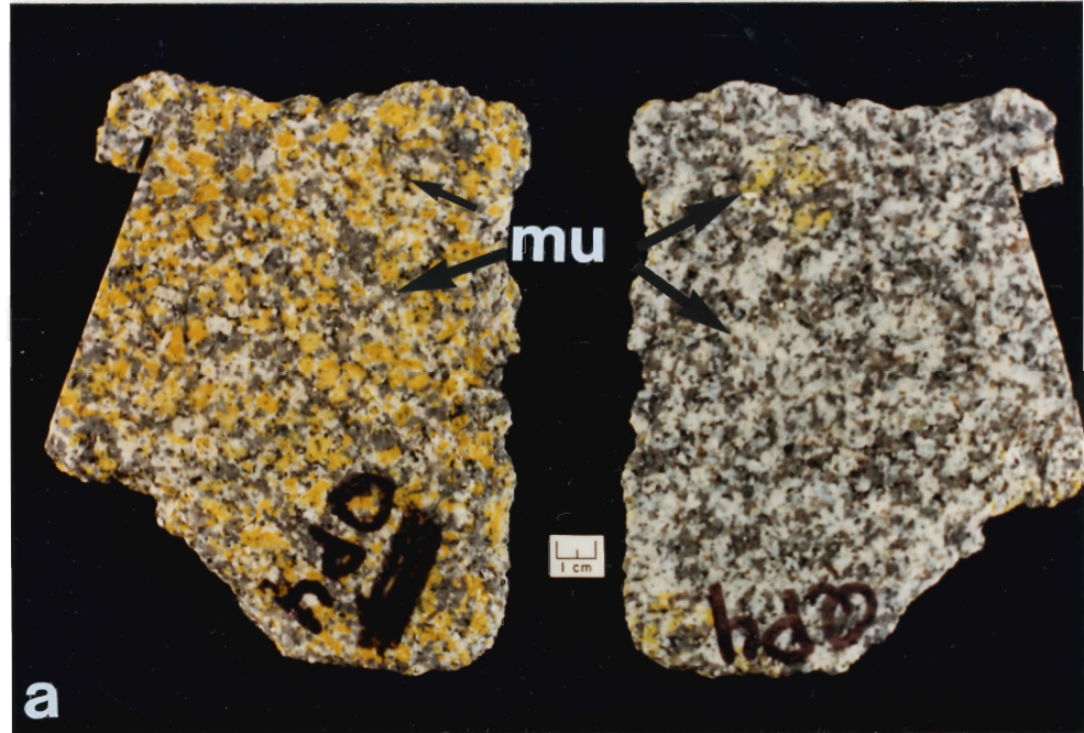
PLATE 2.7. Representative slabs of Unit HCQP4. This unit is fine- to medium-grained, equigranular muscovite-biotite monzogranite. Note in the rocks the easily visible muscovite grains within the matrix (outlined as mu).
