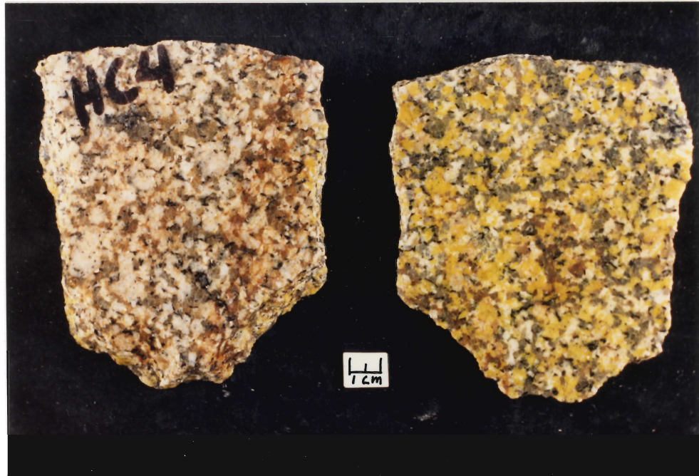
PLATE 2.6. Representative slab of medium-grained (with minor coarse-grained) muscovite-biotite monzogranite of Unit HCQP3.
