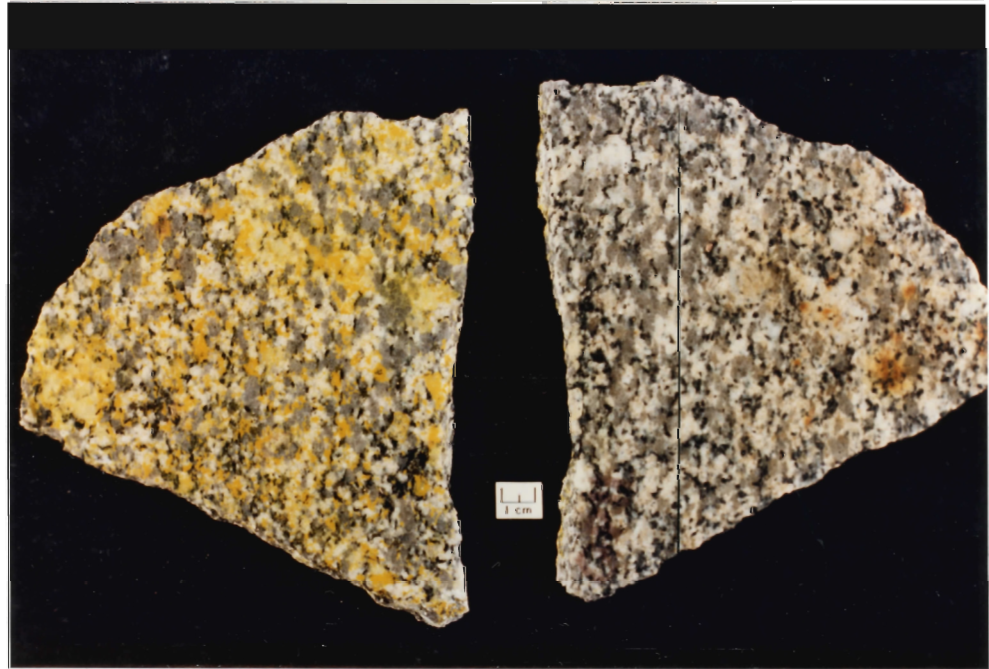
PLATE 2.3. Representative slabs of rocks from Unit HCQP1. Composition is more monzogranitic than Plate 2.2a and b. Notice the alignment of biotite (outlined by the black line) representing a weak mineral foliation discussed in the text.
