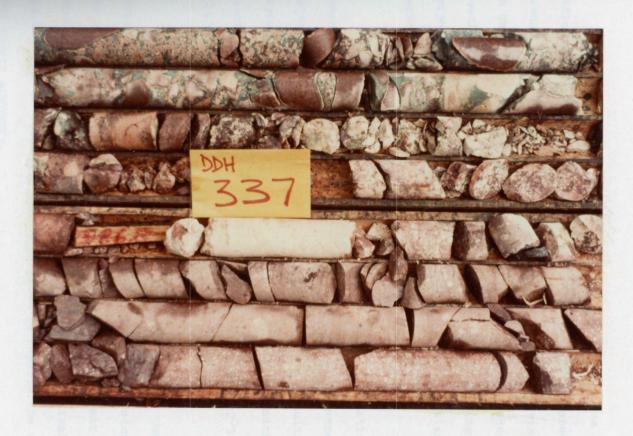
PLATE IV.A.1. Quartz porphyry and overlying talus breccia (DDH 337 - core BQ size).
