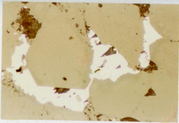
PLATE IV.B.7. Thin section - detail of typical interstitial galena, to show relationship between quartz overgrowth and sulphide fill. (reflected light 275x)
