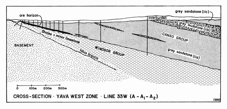
Figure III. 2 Cross-section Through Yava West Zone along line 33w (A-A<sub>1</sub>-A<sub>2</sub>)
