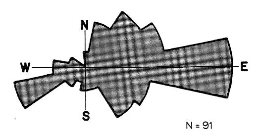
B. Foreset Palaeocurrent directions, Yava West Zone N50°E, 14°NW removed, resulting © 10-25° selected, and uncorrected readings with strikes 30-70° & dips 5-25° omitted.
