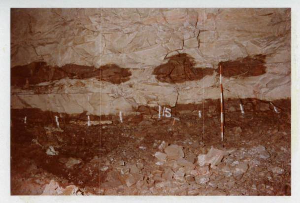
PLATE IV.A.5. Calcareous concretions and bands (weathered rusty brown) in grey mineralized sandstone. (hammer marks Windsor contact, ranging rod = 2 m)
