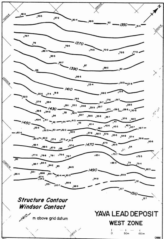
Figure IV.C.11 [Note - Elevations of Windsor/Canso contact shown in metres - last three digits only]
