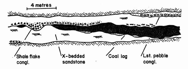
TYPICAL DOWN-DIP WALL SECTION, YAVA MINE, TO SHOW LITHOLOGIC RELATIONSHIP
