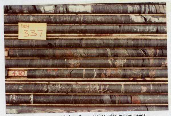
PLATE IV.A.2. Windsor Group shales with gypsum bands (DDH 337 - core BQ size).
