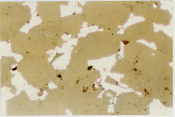
PLATE IV.B.6. Thin section typical interstitial galena in sandstone, - note straight-edged contacts between quartz and galena. (reflected light 175x)
