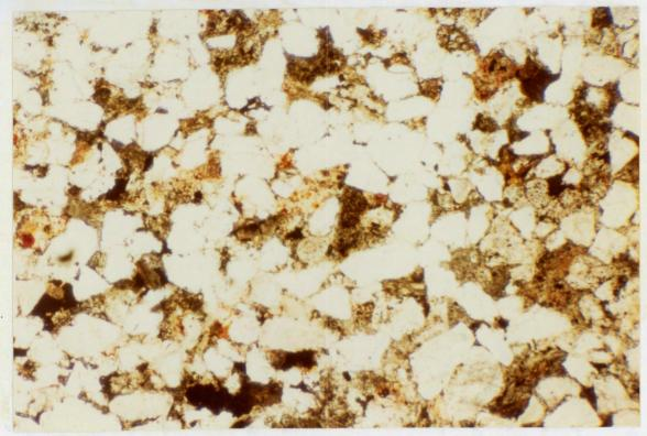
PLATE IV.A.6. Thin section typical host sandstone with clay silicate cement. (PPL 45x)
