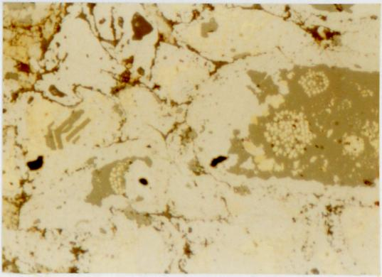
PLATE IV.B.10. Framboidal pyrite in a sphalerite groundmass, infilling plant cells, surrounded and replaced by later galena.
