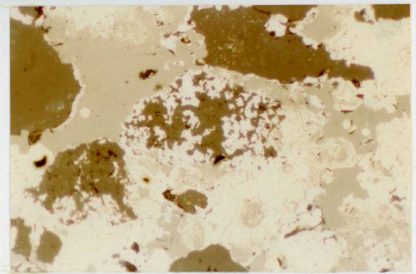
PLATE IV.B.9. Sulphide assemblage adjacent to coal material, showing zoned pyrite and sphalerite, and later galena mineralization.
