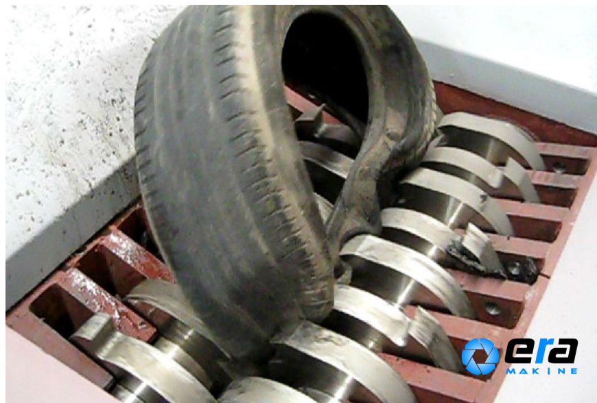
Figure 1.3 Tire shredding blades (“Era Makine” n.d.)
