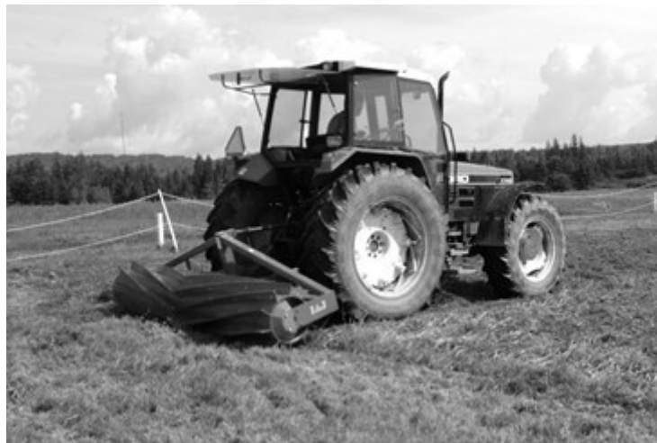
Figure 2.1. Crop roller used to no-till terminate hairy vetch/oat Gmr (I and J Manufacturing, Gordonville, PA). The barrel of the roller is filled with water to create more downward force.
