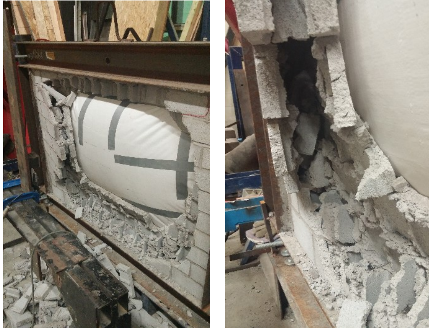
Figure 4.38 Out-of-plane failure mode for specimen IF-S-CC
