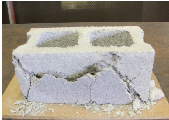
Figure 4.2 Typical failure mode - shear failure in CMUs
