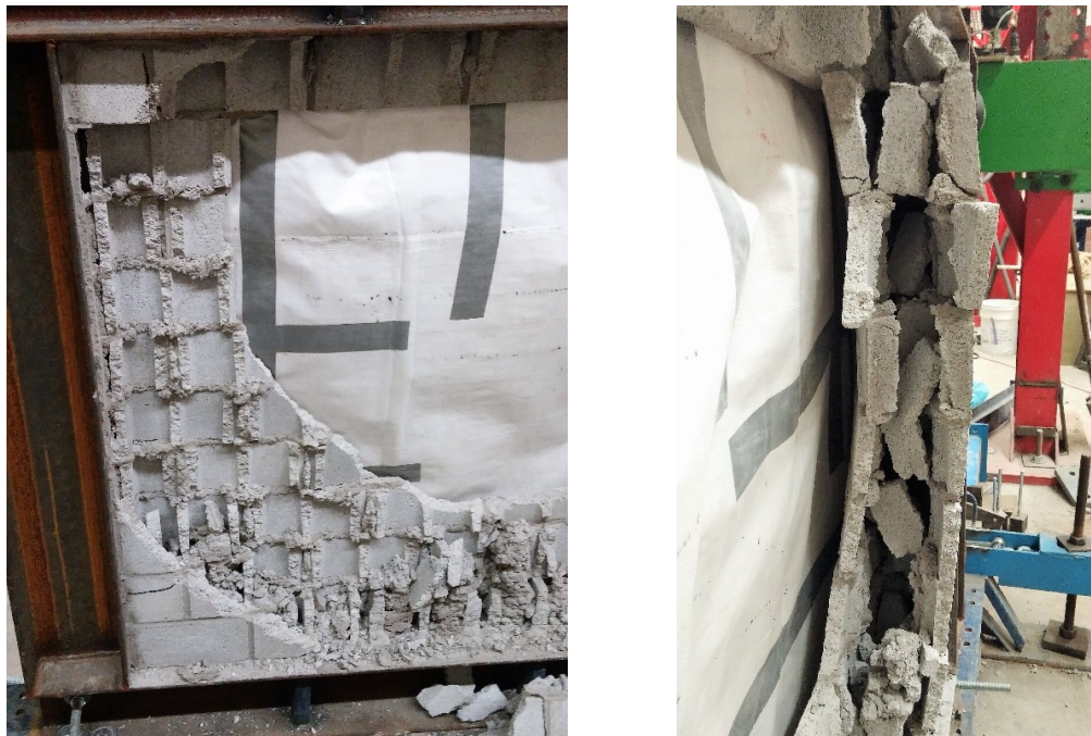
Figure 4.12 Faceshell separation due to web shear failure on specimen IF-S-SW
