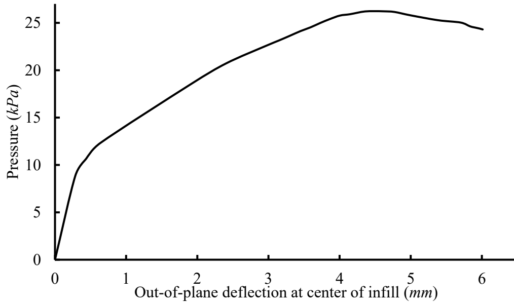
Figure 4.21 Pressure vs. displacement curve for out-of-plane loading on specimen IF-S-D1
