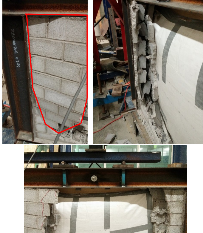
Figure 4.43 Specimen IF-S-VL failure pattern after out-of-plane loading
