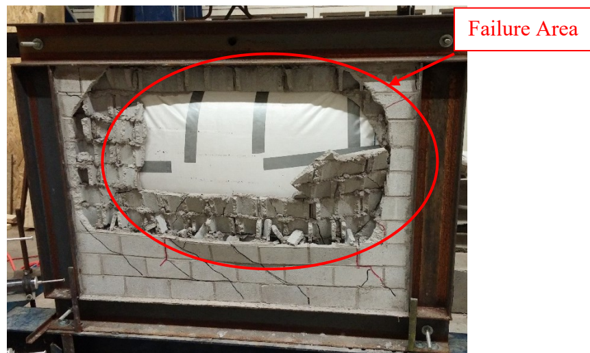
Figure 4.32 Out-of-plane failure mode for specimen IF-S-D2
