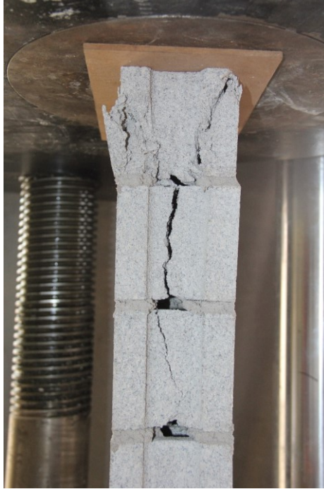
Figure 4.4 Typical failure mode of masonry prism test
