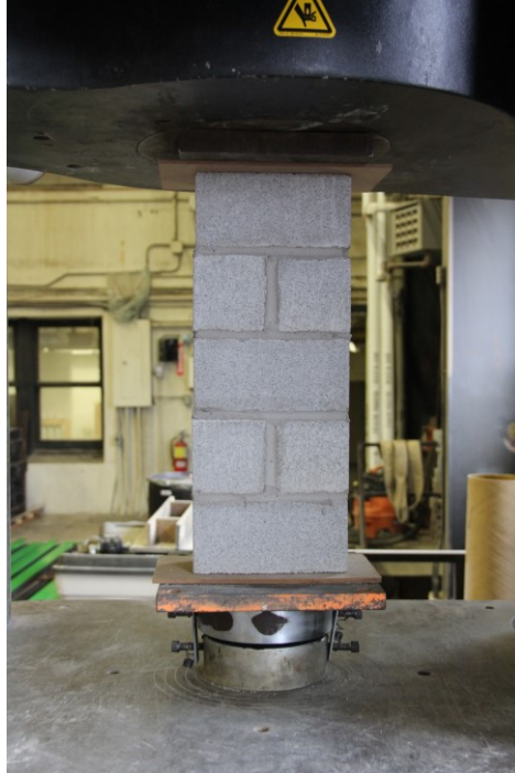
Figure 3.15 Compression test for masonry prisms
