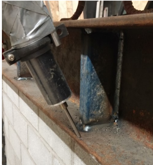
Figure 4.13 LVDT 6 measuring top beam flange deflection
