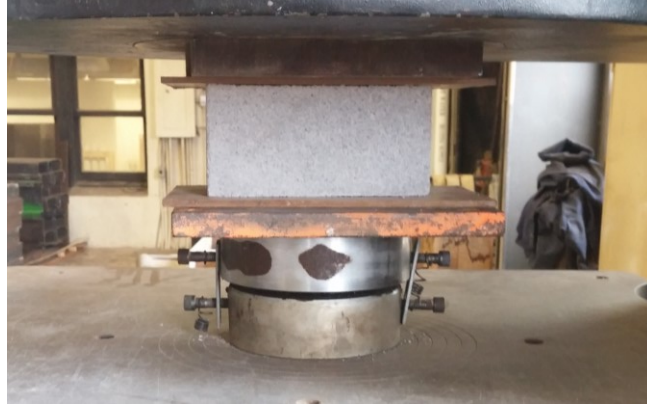
Figure 3.13 Compression test for CMUs
