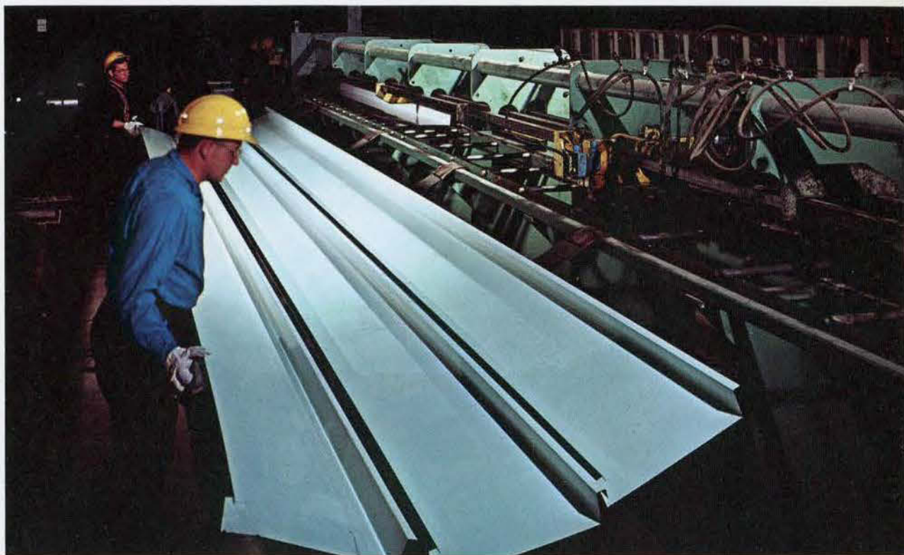
Production inspection at Armco Drainage & Metal Products of Canada Ltd. new roll-forming equipment ↑
