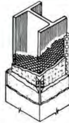
Vertical columns are fireproofed and finished with gypsum plaster over self furring metal lath. Recesses between column flanges provide excellent ducts for service pipes.
