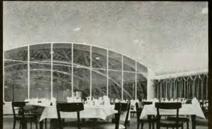
The dining room of a Toronto gentlemen's Club has an Asbestospray ceiling for acoustical correction. Architect: Basil G. Ludlow, Toronto General Contractor: W. B. Sullivan Construction Ltd. Toronto Asbestospray by: David McFarlane & Assoc. Ltd. Toronto.
