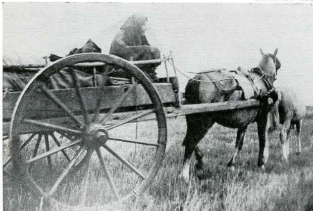
Red River cart. The original version of this utility conveyance of the prairies was constructed entirely of wood.
