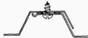
5, two synthetic rubber tapes reinforced with fabric are held under pressure on either side of the sheet metal screw. Such tape provides a very effective and easily applied seal.
