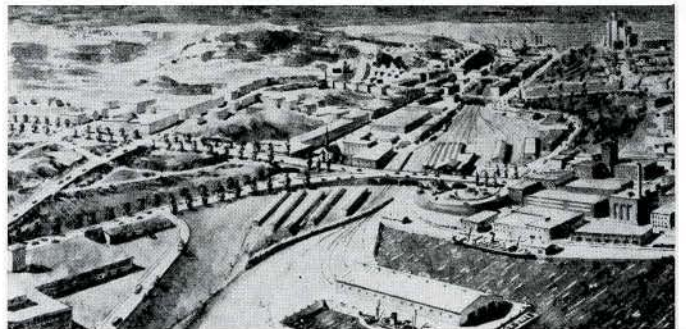
Aerial view of the central valley, showing proposed viaduct, traffic separation, northern access road. Left centre is Fort Howe Park extended downhill to replace a slum.
