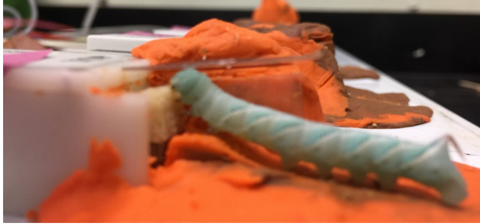
Figure 2.1 Picture of the force transducer setup utilized in the caterpillar feeding experiments. Half of the plasterine normally around the setup has been removed to show the position of the caterpillar.
