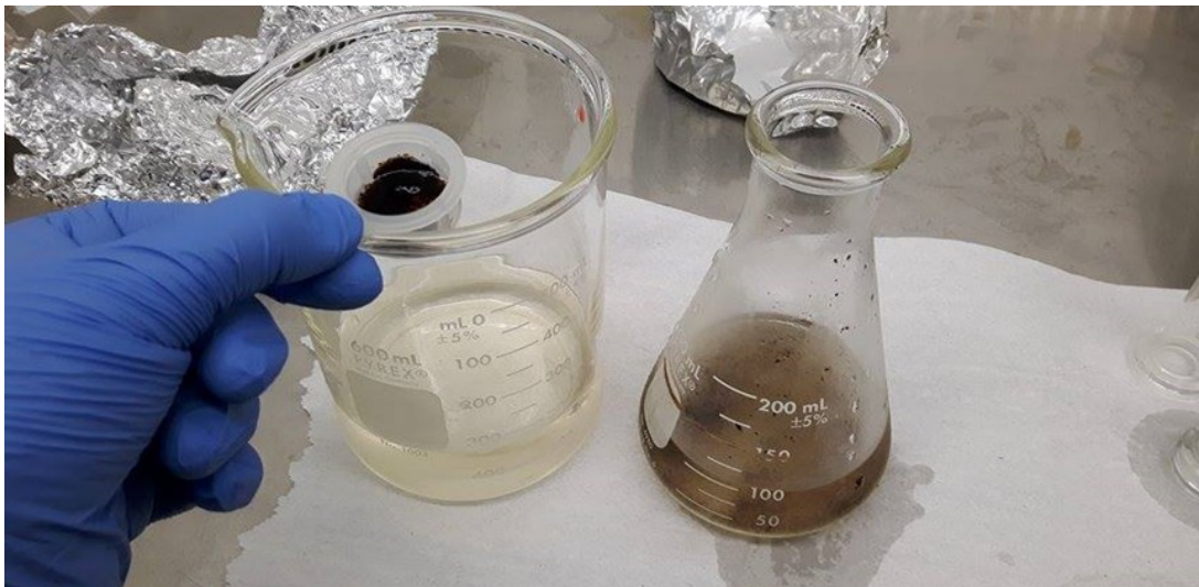
Figure 4.1. A tributary sample undergoes an initial filtration to remove debris larger than 70 \mu\text{m} prior to vacuum filtration for cyanobacteria isolation.
