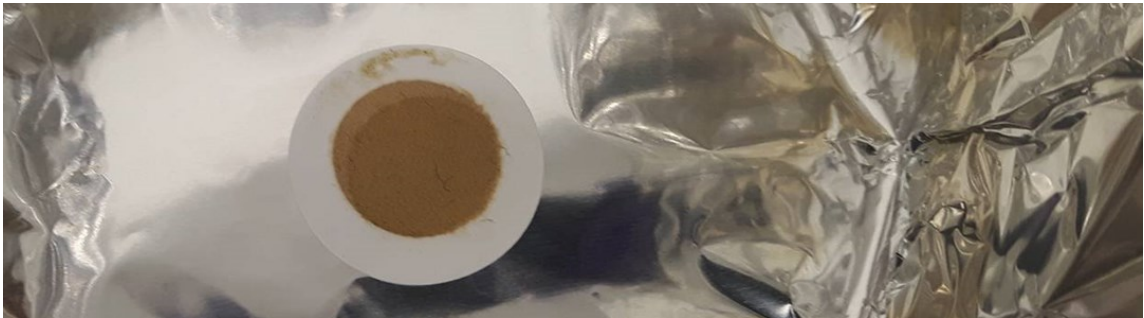
Figure 2.5. Example of a PES filter post vacuum filtration being prepared for storage.
