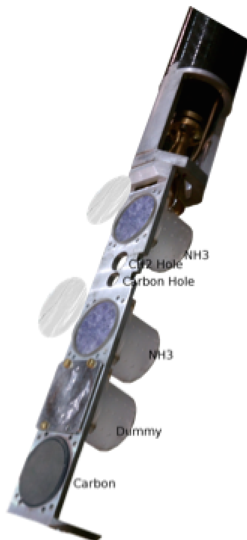
Figure 2.12: This figure shows the vertical orientation of the target insert shown in Figure 2.11 along with the placement of each of its target cells. In particular, it highlights the locations associated with the top and bottom \text{NH}_3 targets, the carbon and dummy targets, as well as the \text{CH}_2 target and the position of the carbon holes [73].
