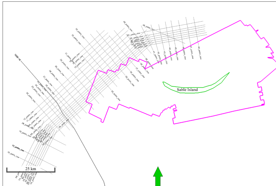
Figure 3.4: Location of 2D seismic (grey lines) in relation to the 3D Sable MegaMerge (purple polygon) and the 2D regional NovaSpan line 1600 (longer black line).
