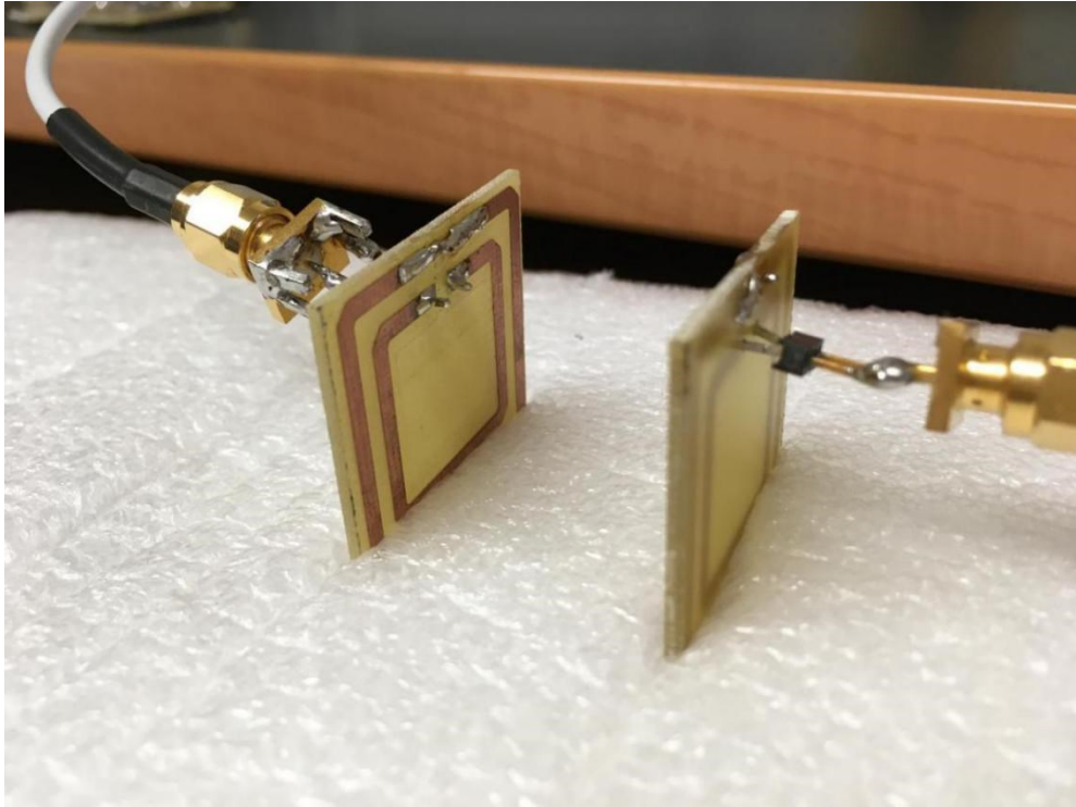
Figure 4-6: The conventional WPT system and its test setup.
