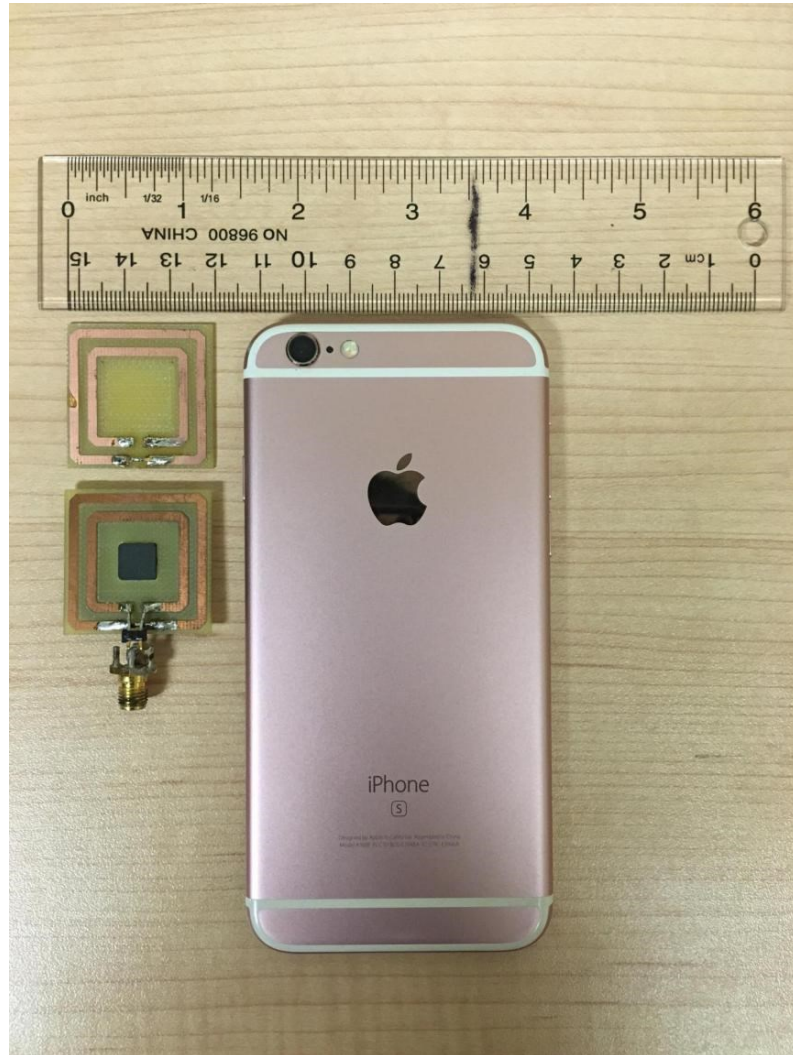
Figure 4-8: The conventional and the proposed WPT receivers in size comparison of iPhone 6s.
