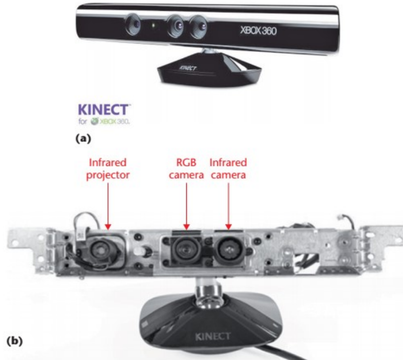
Figure 2-1. The structure of Microsoft Kinect sensor [12]
