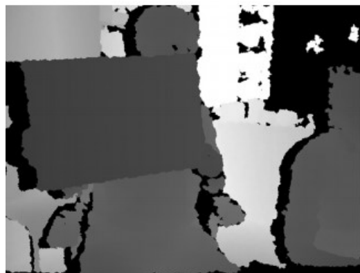
Figure 2-2. Depth image of the Kinect sensor [12]
