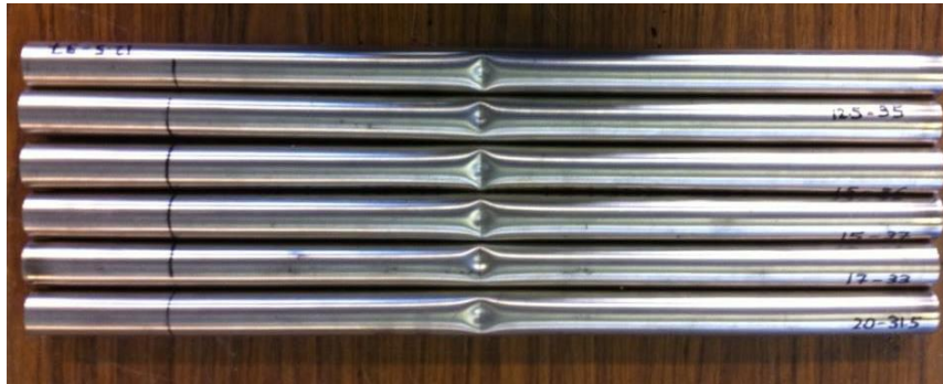
Figure 5.10 Final shapes of the pipes tested under symmetric cyclic bending loads
