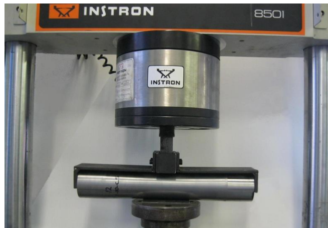
Figure 3.4 Test set up used for generating the indentation
