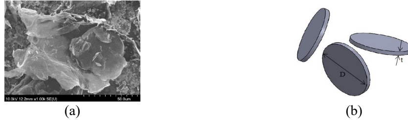
Figure 6-3. GNP nanoparticle (a) SEM image; (b) schematic of the idealized GNP (Ahmadi-Moghadam and Taheri 2014)
