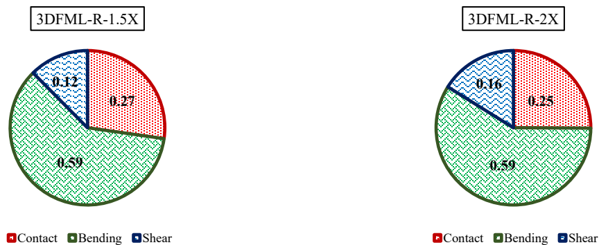
Figure 8-24. Fraction of absorbed energy by contact, bending and shear deformations of the baseline-3DFMLs impacted by two different sizes of impactors
