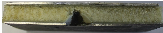
Figure 3-19. Typical failure pattern seen in 3DF-FMLs at the second-stage impact loading
