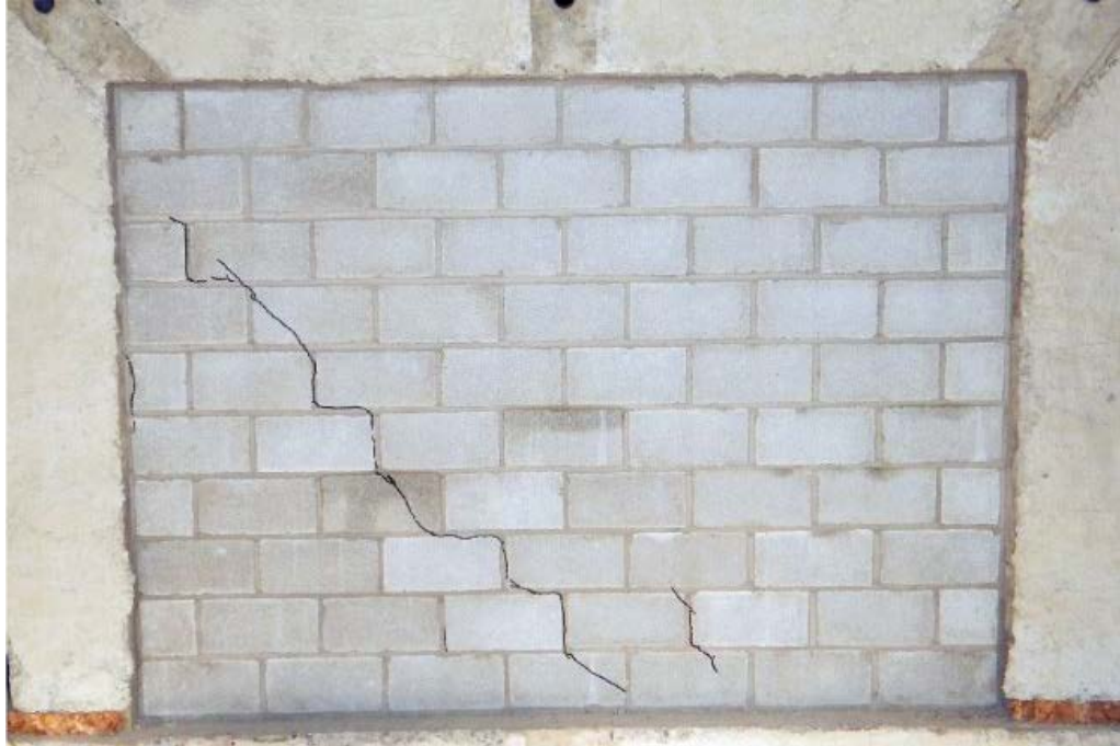
Figure 4.19 Prior In-Plane Damage for Specimen IF-D1 (Sepasdar 2017)
