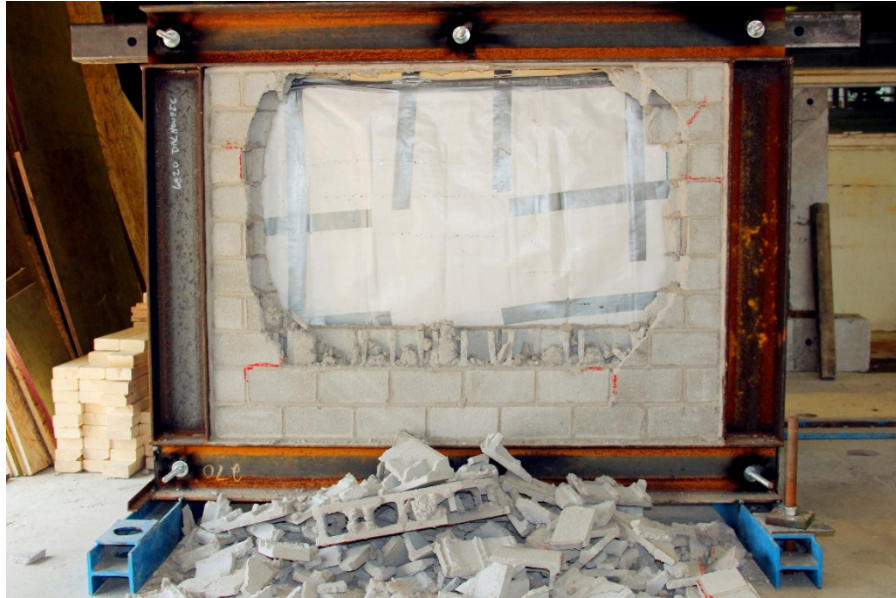
Figure 4.40 Failure Mode of Specimen IF-S on Leeward
