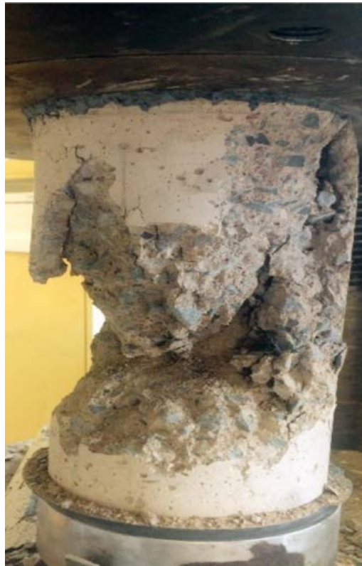
Figure 4.6 Typical Compressive Failure of Concrete Cylinder
