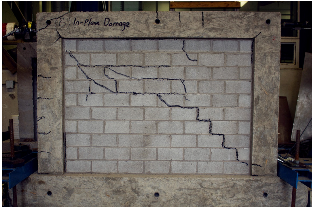
Figure 4.18 Prior In-Plane Damage for Specimen IF-RC-ID
