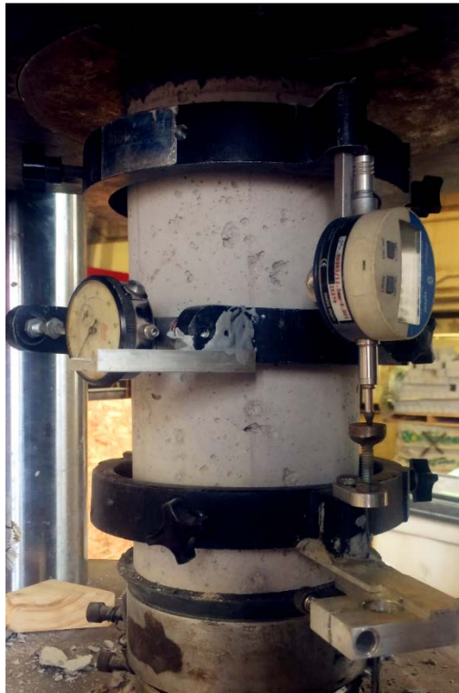
Figure 3.32 Compression Test Set-up for Concrete Cylinder
