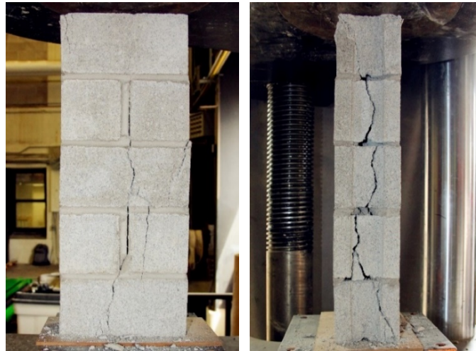
Figure 4.5 Typical Compressive Failure of Masonry Prisms
