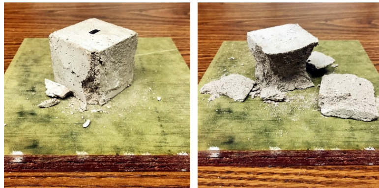
Figure 4.3 Typical Compressive Failure Mode of Mortar Cubes
