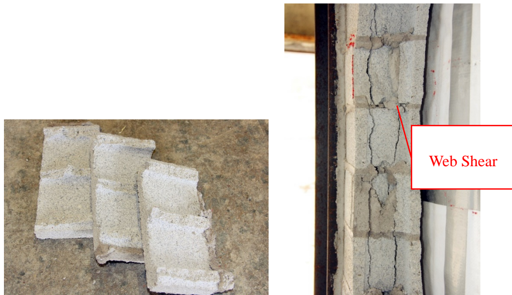
Figure 4.41 Web Shear Failure of Masonry Units for Specimen IF-S
