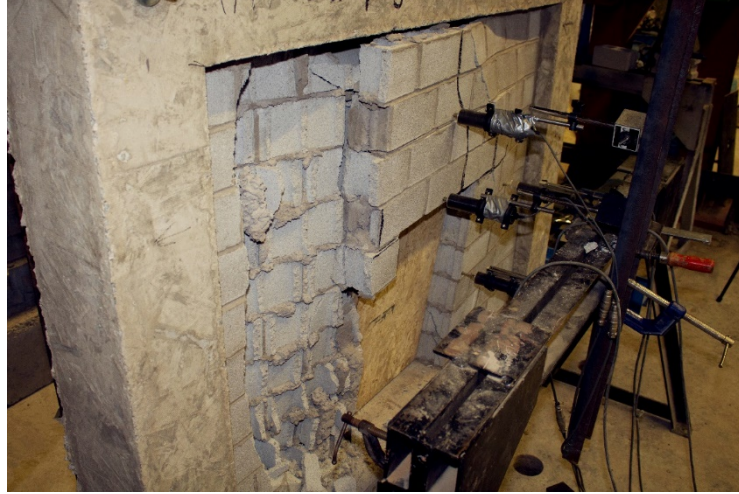
Figure 4.10 Failure Mode of Specimen IF-RC-DO on Leeward
