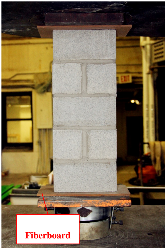
Figure 3.31 Compression Test Set-up for 5-Course Masonry Prisms
