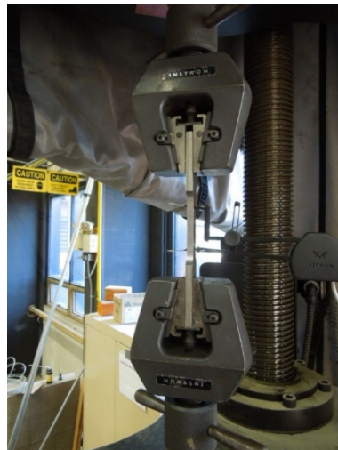
Figure 3.36 Tension Test Set-up for Steel Frame Coupons
