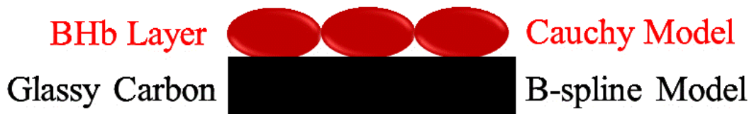
Figure 6.5 A diagram illustrating a two-layer model used for spectroscopic ellipsometry to determine the thickness of the BHb layer.
