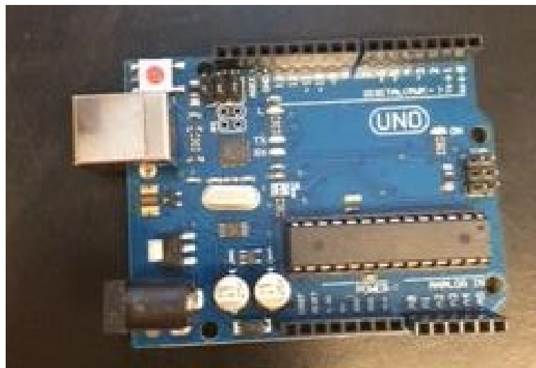
Figure A-4. An image of the Arduino Uno Rev3. This device was used to control the pulsing of LED lights. A script was written in Arduino IDE software to get the desired pulse.
