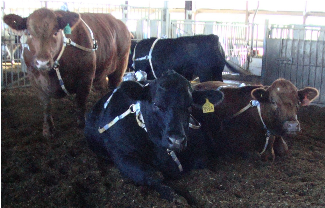
Figure 3.1 Polar system and custom leather harness equipped on steers using identical equipment as used in this research trial. The leather harness consisted of a chest strap containing the Polar electrodes and transmitter, a neck strap and four horizontal straps to secure the device.
