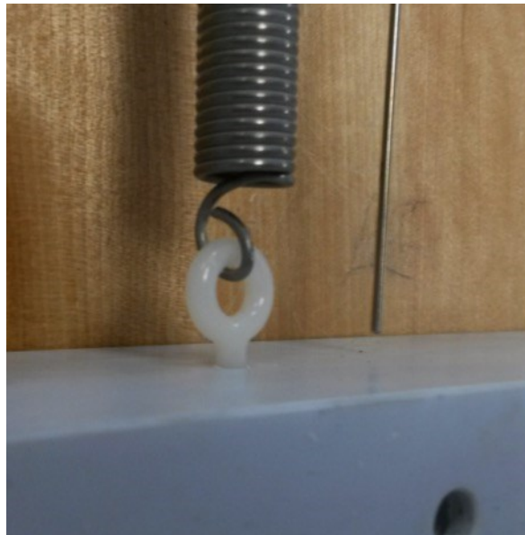
Figure 3-9: Close-up view of the crimped spring-wire attachment used to secure spring-bottoms to the eyebolts in Marks I and II.
