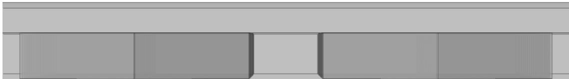
Figure 4-16: Lateral-view from Figure 4-14 showing only the HTF channel. Note the bottom layer consists only of the interstices remaining around the aluminum pattern elements in Figure 4-15 (i.e., embossed pattern).
