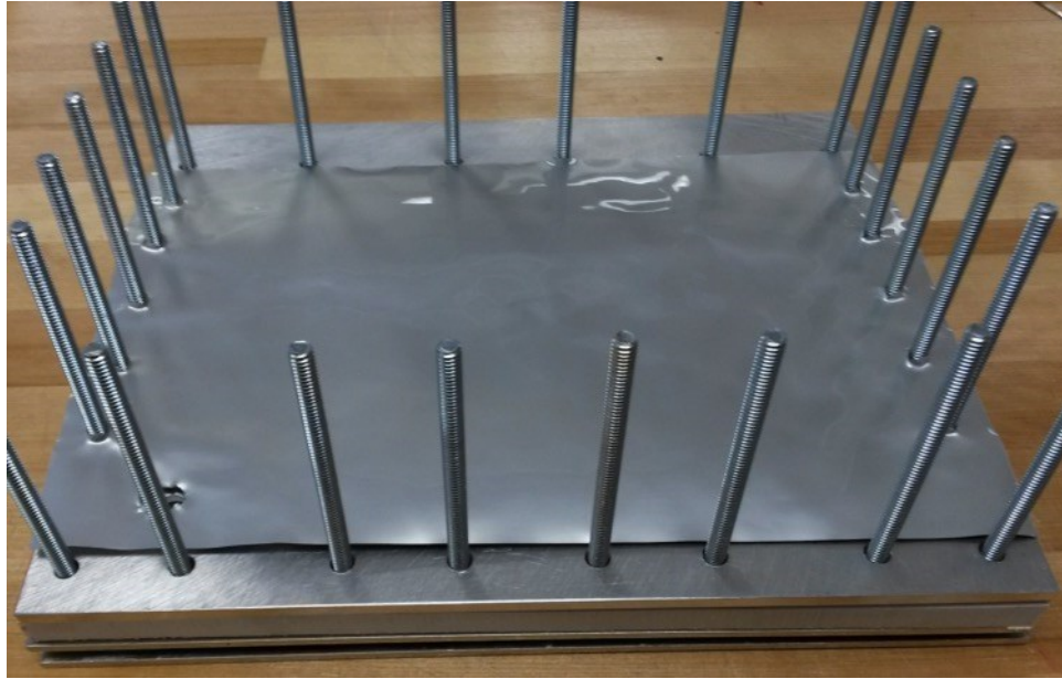
Figure 3-16: Inside-facing view of the complete heat exchange plate assembly for Mark III, showing the aluminized barrier film used to isolate the aluminum flow plate from the SAT PCM.
