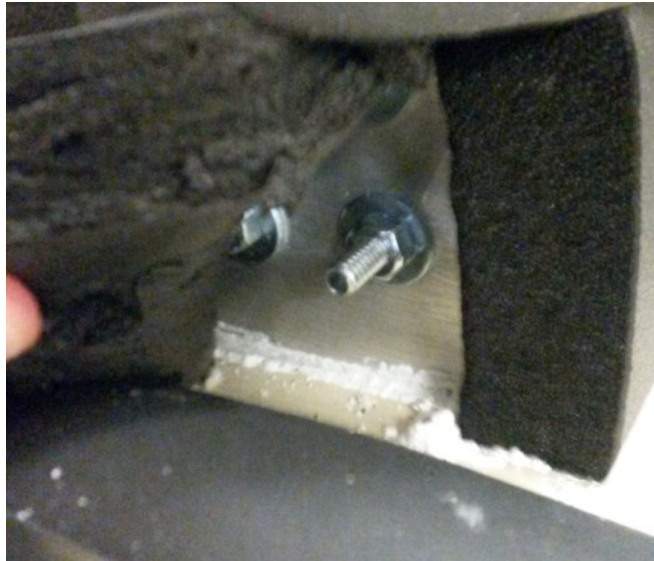
Figure 3-29: Traces of sodium acetate, either anhydrous or trihydrate, found at the bottom edge of the Mark II heat storage cell after 37 repeated charge-supercooling-discharge cycles in the circulated HTF experiments shown in Figure 3-23.
