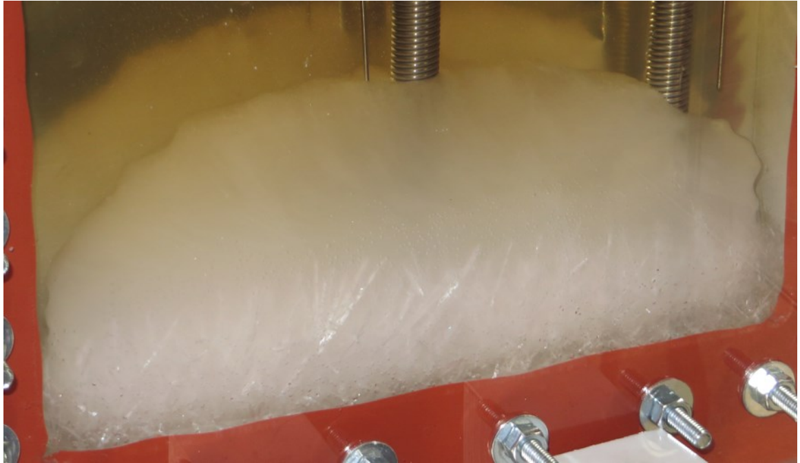
Figure 3-33: Solid SAT PCM remaining near the bottom of Mark I (early model with only two springs) while charging in the environmental chamber. The reflection of the solid PCM produced on the aluminized film shows that more solid SAT remains near the PC sight-glass than toward the aluminized film.
