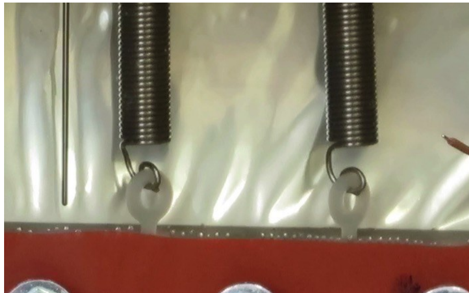
Figure 3-37: Image capture from HD video taken at the beginning of a nucleation triggering experiment using Mark I. The SAT PCM was fully dissolved and supercooled to 22\text{ }^{\circ}\text{C} with no signs of anhydrous SA present. The spring-nucleation triggers shown here correspond to those shown in Figure 3-36.
