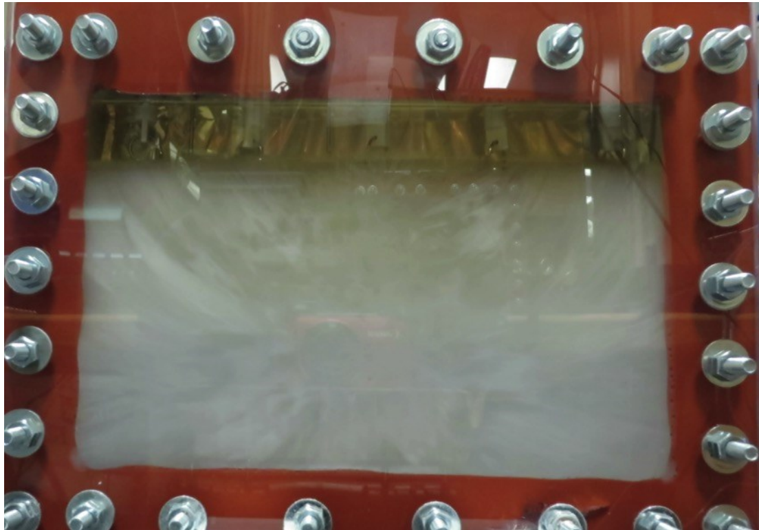
Figure 3-69: Mark I heat storage cell exhibiting solution stratification after repeated charge-discharge cycles with full dissolution. The solidified room-temperature state is shown for ease of visualization. The solution was separated into a smaller, upper stratum containing only dilute solution ( w_{SA} \leq 0.32 ) and a larger, lower stratum containing a concentrated mixture of SAT and water ( 0.532 \leq w_{SA} \leq 0.603 ).
