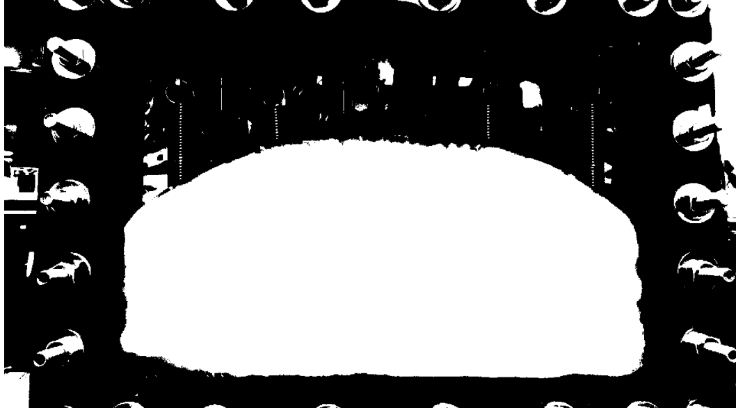
Figure 3-56: Binary image conversion from the grayscale image in Figure 3-54 for pixel intensity \geq 130 .
