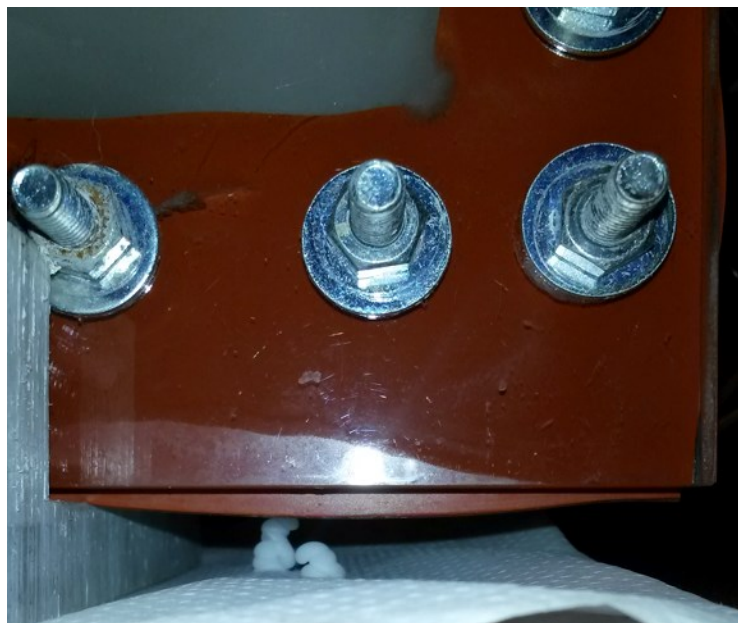
Figure 3-27: A deposit of solid SAT found directly underneath an eyebolt port underneath the Mark I heat storage cell at the end of a 167 day long-term supercooling experiment.
