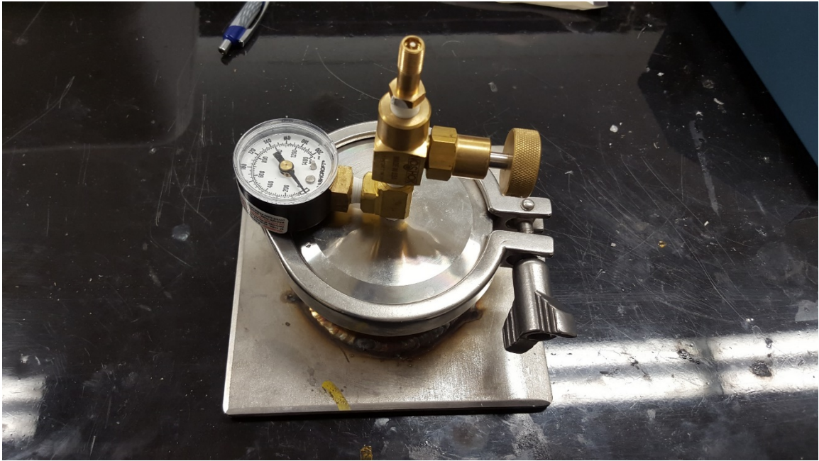
Figure 2.2: Pressure chamber for high pressure curing of Platsil
