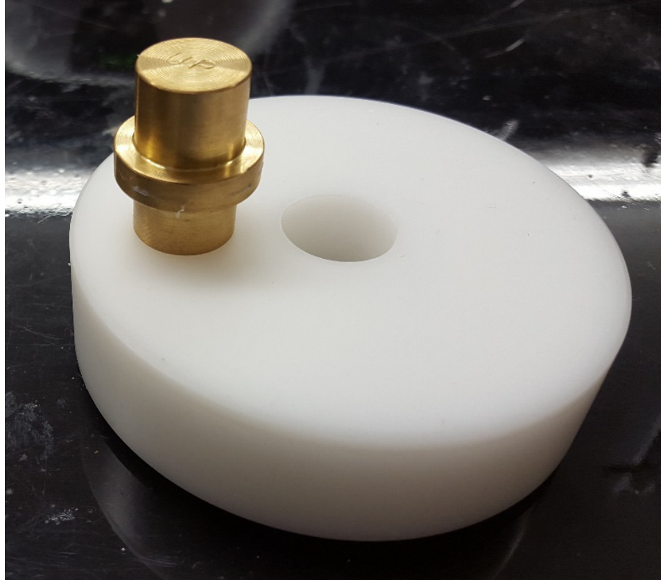
Figure 2.29: Teflon mould with brass insert
