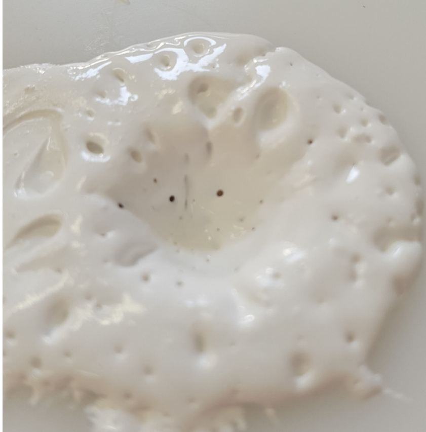
Figure 2.17: Bubble-filled, ZnO doped Silicone
