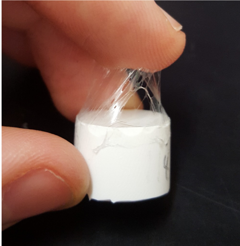
Figure 2.20: FastelTack Sil PSA delaminating from surface of Sylgard 184
