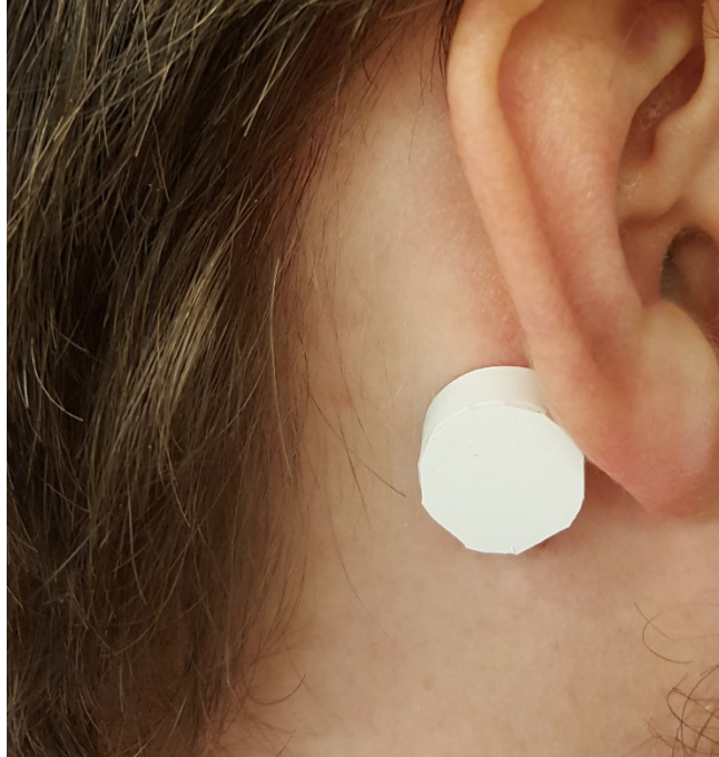
Figure 2.23: Final Dry Coupling Design Attached to Head on Mastoid Tip
