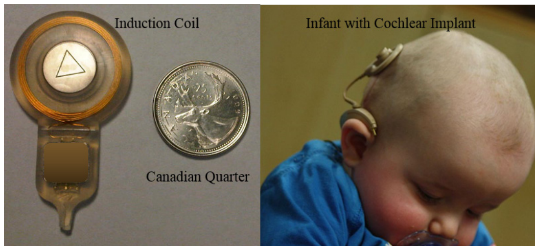
Figure 1.3: EM Induction Coil for Cochlear Implant
