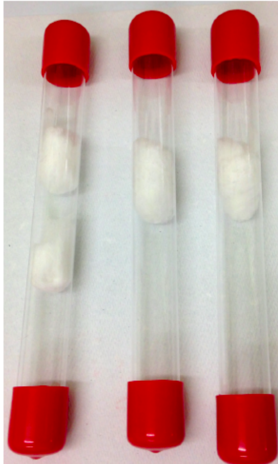
Figure 2.9. Three breath collection tubes with caps. The breath collection tube on the left, which will be used to collect the target breath sample, holds two cotton balls so that after sample donation, one can be removed and used as the sample stimulus.
