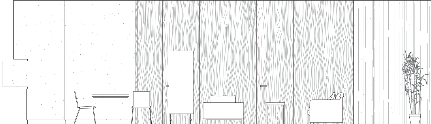
Figure 87: Interior elevation B of the typical cocoon. Note that the entire apartment is on one level, without threshold on the ground all the way to the balcony for easy access to wheel chair users. The doors slide easily. These enclose the "walking closet" and the bathroom.
