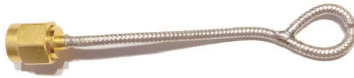
Figure 3.1: Shielded magnetic field probe, before wrapping in an insulator to allow safe probing of any area of the device under test.
