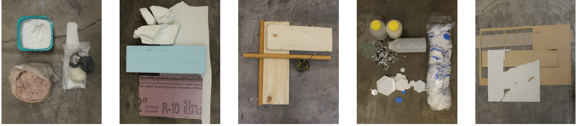
Image 63: Salvaged model material: clays/plasters, extruded foams/boards, wood, plastics/acrylics, card.
