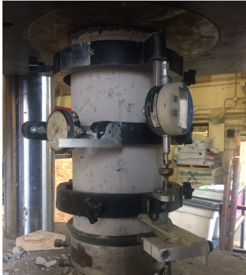
Figure 3.30 Compression Test Setup for Concrete Cylinders
