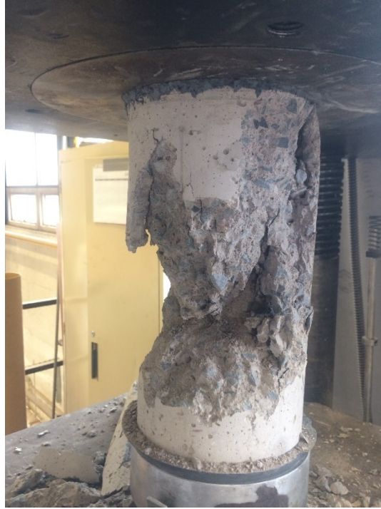
Figure 4.6 Typical Failure Mode of Concrete Cylinders
