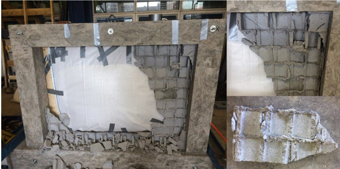
Figure 4.34 Out-of-Plane Failure Mode of Specimen IF-D2
