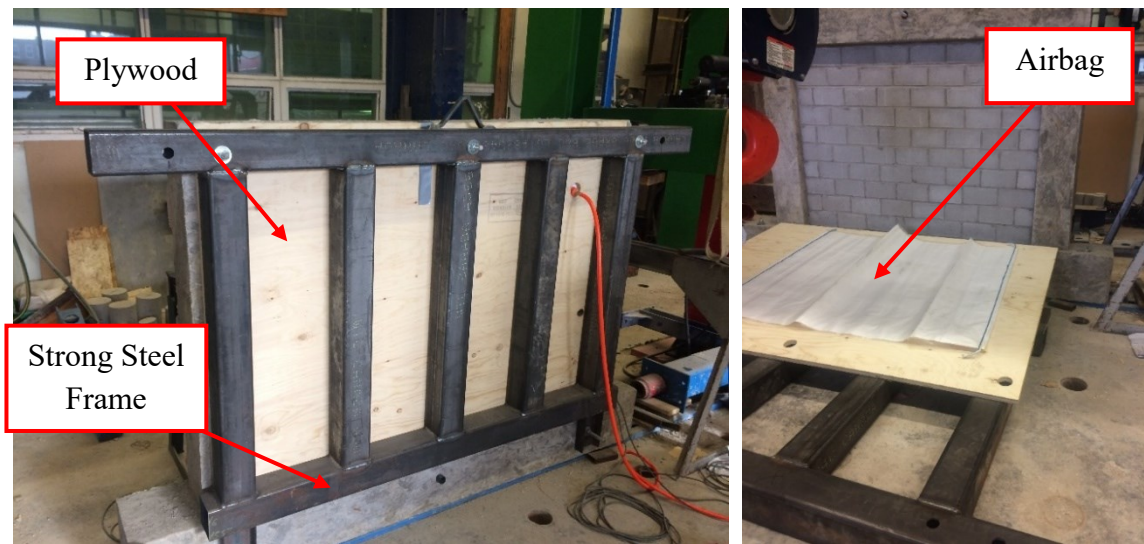
Figure 3.14 Out-of-Plane Test Setup
