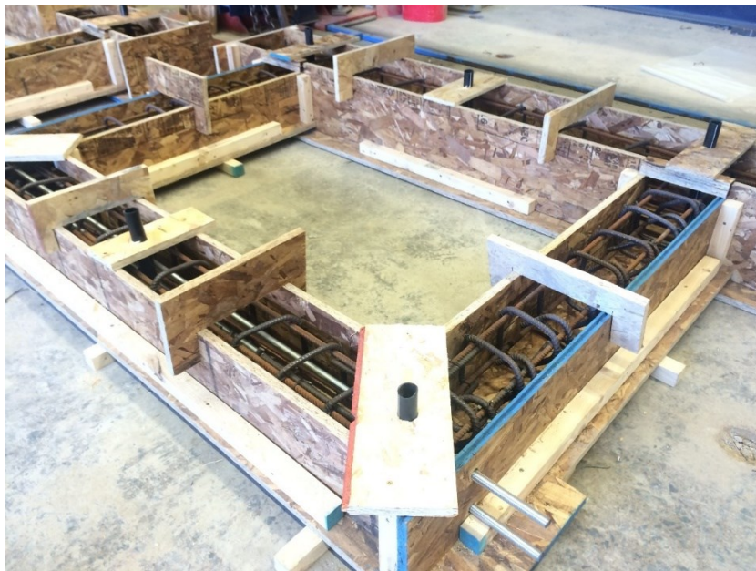
Figure 3.9 Frame Specimen Ready for Pouring Concrete
