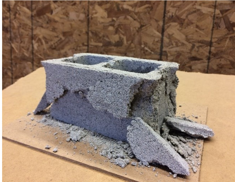
Figure 4.2 Typical Failure Mode of the CMUs
