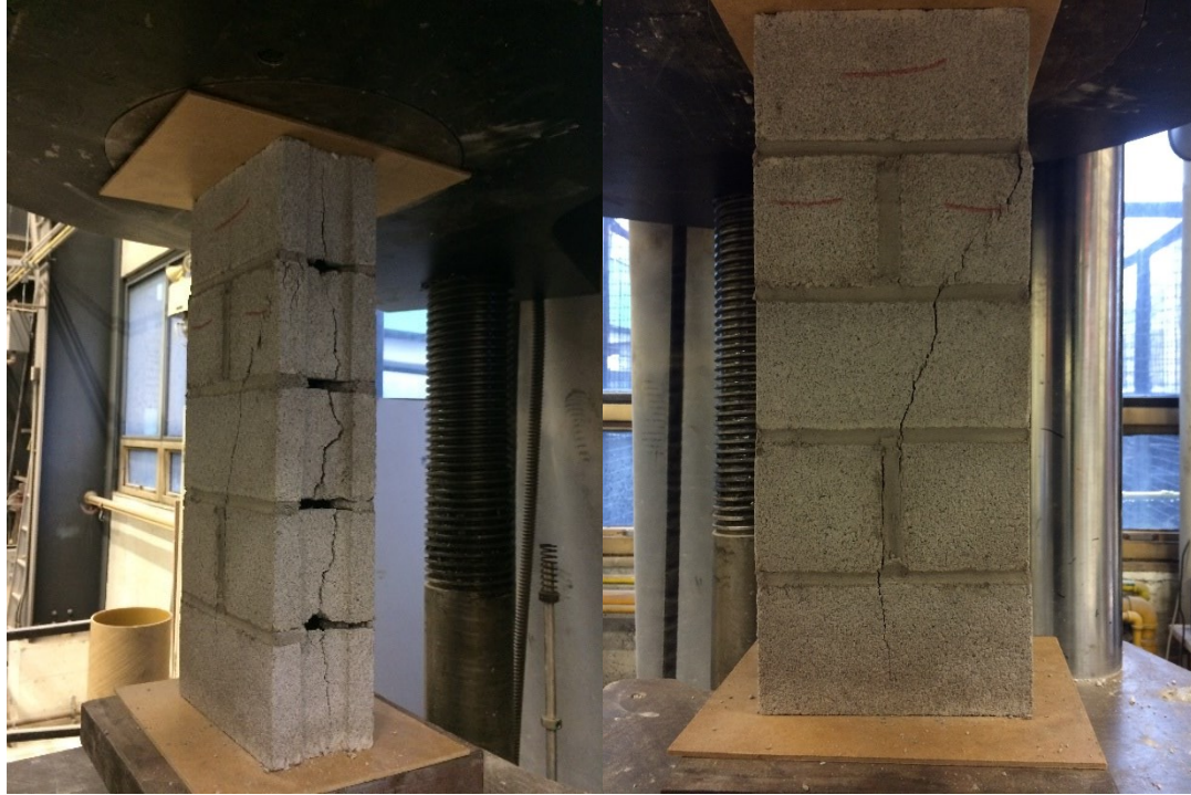
Figure 4.5 Typical Failure Mode of Masonry Prisms
