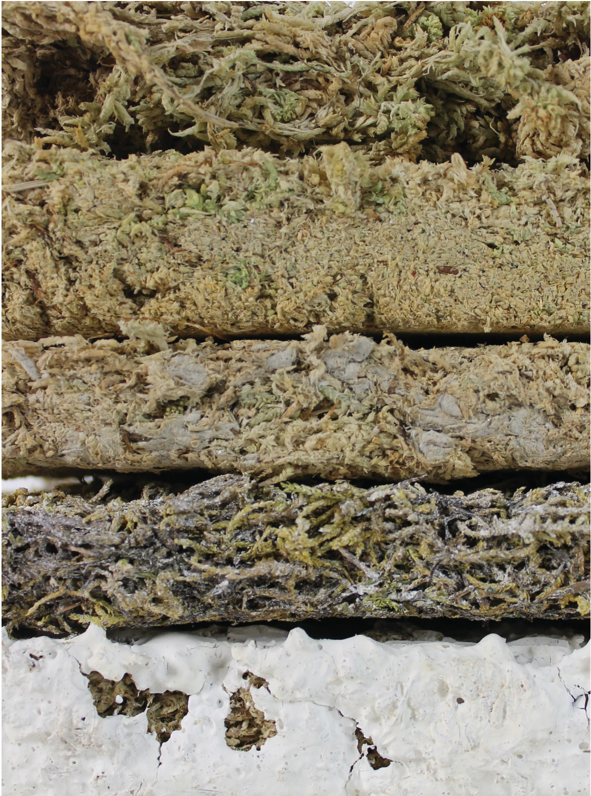
Experimenting with sphagnum moss as an alternative to rigid insulation. From top to bottom: (1) lightly compressed (2) pulped and compressed (3) pulped w/ shredded paperboard and compressed (4) pulped w/ calcium stearate and compressed (5) pulped, compressed, dried and dipped in calcium stearate.
