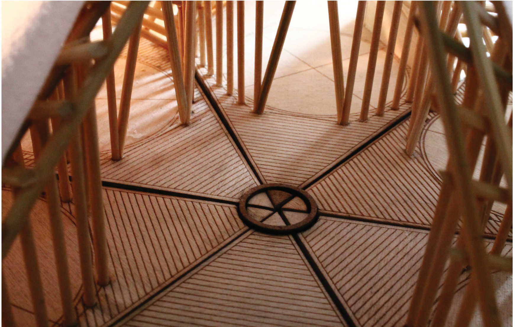
3D physical model. Embedded fireplace ring connection.
