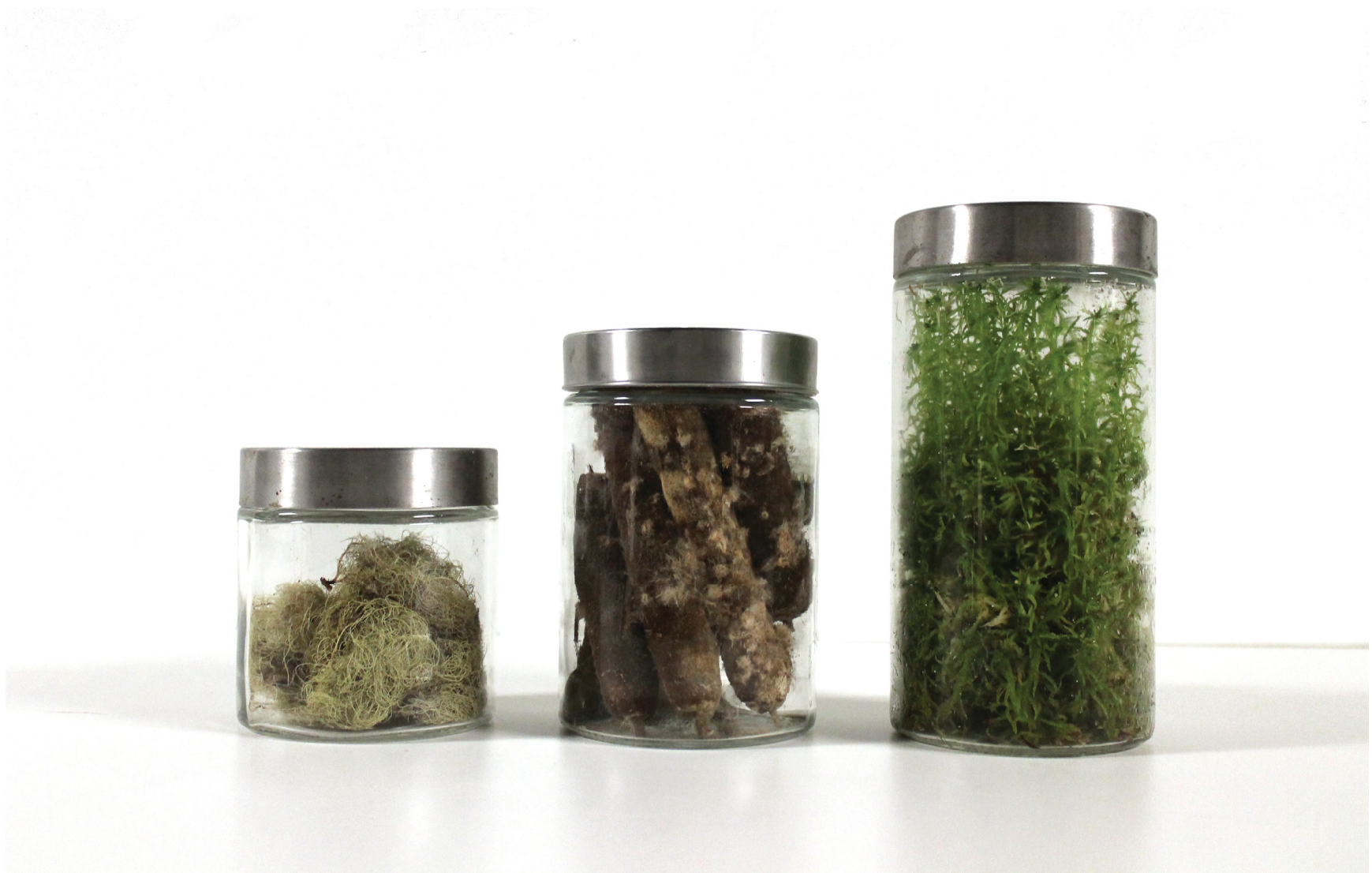
Experiments in natural insulating materials. From left to right: Usnea (old man's beard), cattail (bulrush), and sphagnum moss.
