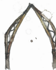
Bentwood truss arch (design by Richard Kroeker)
