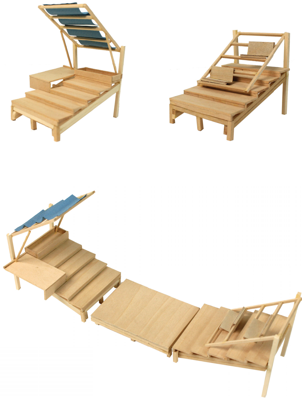
fig. 31.0. One module unit. Both awning conditions are shown in model. Original model scale at 1:50.
