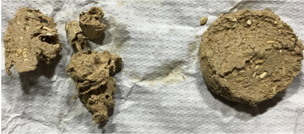
Figure 38 - Left to right, non-sonicated dried sludge versus sonicated sludge.
