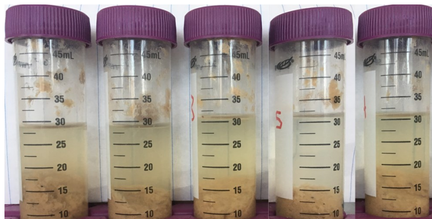
Figure 41 - WAS samples with ranging acid (93% sulfuric acid) addition volumes from 0 to 0.20 mL (left to right, 0.05 mL increments)
