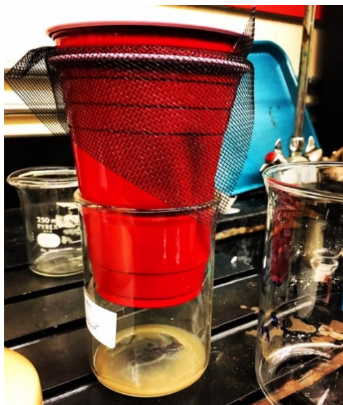
Figure 37 - Handmade small scale pressure exertion design using red Solo™ cups and screen mesh.
