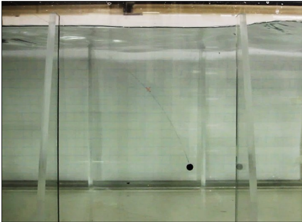
Figure 3.11: Tow cable and towed sphere.
