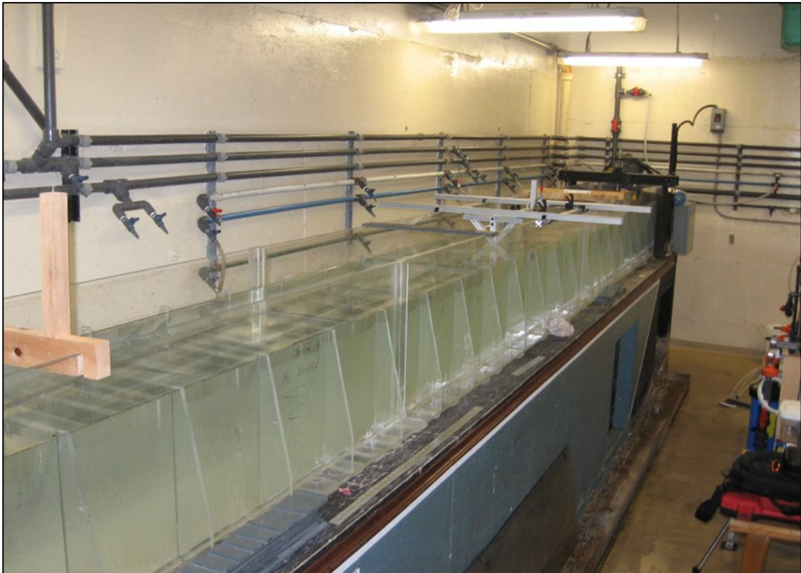
Figure 3.8: Dalhousie Aquatron lab's flume tank with aluminum camera mounting frame.
