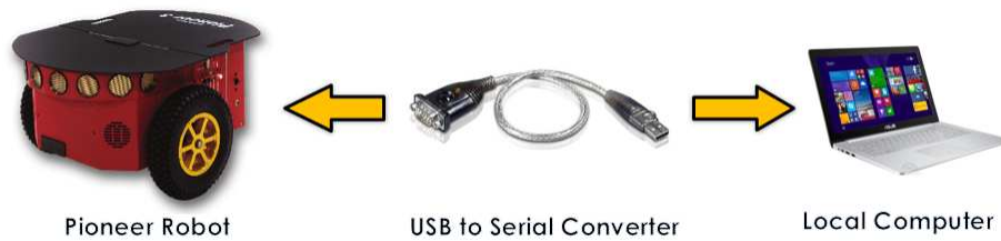
Figure 5.2: Connection between Pioneer Robot and local computer
