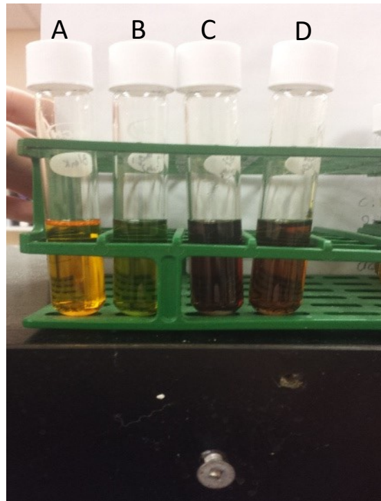
Figure 5-1: Comparing colour changes in closed reflux chemical oxygen demand (COD) test tubes between the blank (A), raw wastewater (B), 100% permanganate:COD (C) and 50% permanganate:COD (D).
