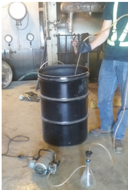
Figure 3-1: Wastewater collection method using a vacuum pump, vacuum flask and modified pipette.
