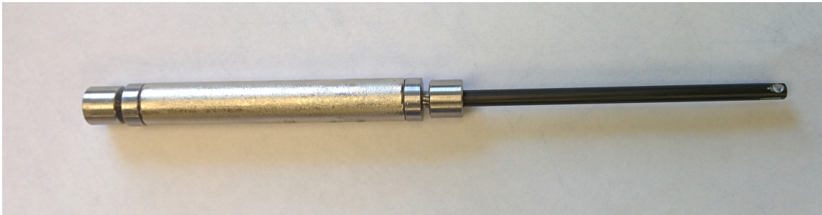
Figure 2.6: 3 inch magnet with piston heads (no seals)
