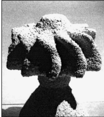
Figure 2-23. Investment casting mould for TiAl turbine wheel [20].
