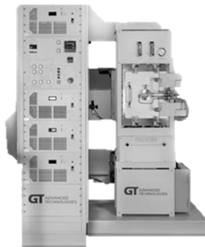
Figure 2-30. A typical SPS chamber and power unit (Series 20, GA-Technologies).
