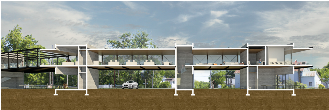
Sectional perspective - Creative hub spanning over Foundry Road and the recreational pathway. The solid concrete cores contain the workshops, amenities and vertical circulation while the collaborative workspaces are located within a glassy elevated space. (The workshops are separated from the workspaces due to noise and debris).
