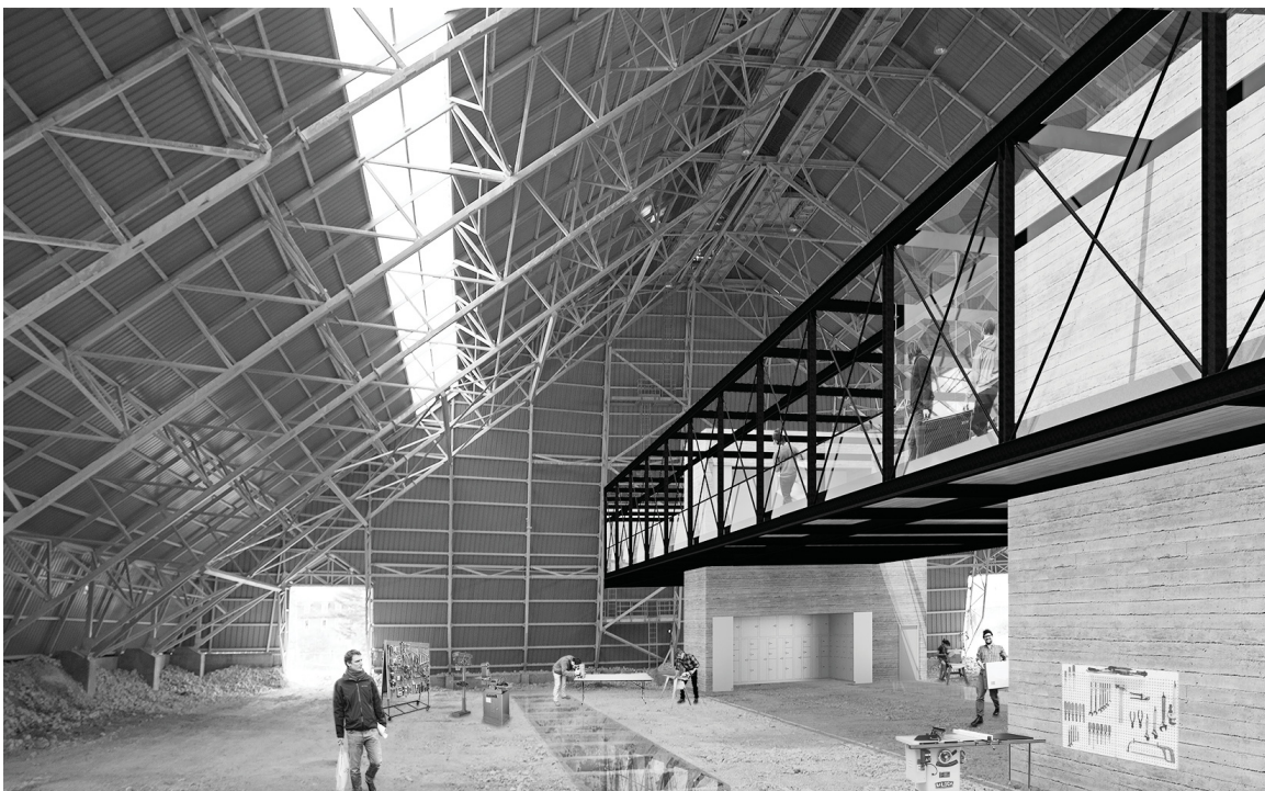
Gypsum shed interior perspective - Workshop program expanding into abandoned industrial infrastructure. The elevated bridge creates a space separate from the workshop floor for leisure and different vantage points and the solid cores house storage space, private amenities and circulation.
