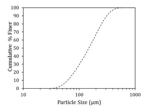
Figure 28: Particle size distribution for the PA7055 powder.
