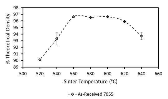
Figure 16: Baseline sintering response of PA7055 (As-received powder; all samples CIPed at 400 MPa).
