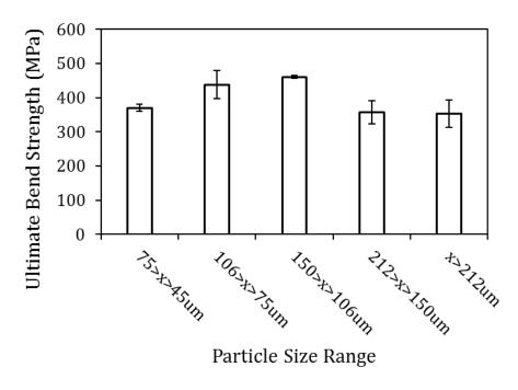
Figure 39: Effect of average particle size on the ultimate bend strength of PA7055 specimens consolidated at 500°C (Type II; 120s hold time).
