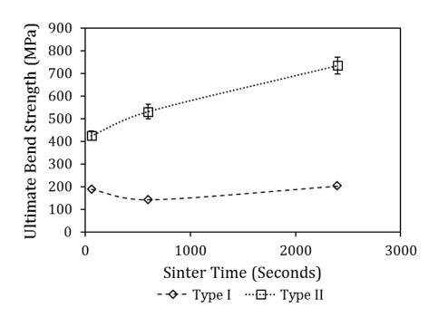
Figure 35: Effect of sintering time on the UBS of PA7055-T76 specimens consolidated at 500°C.
