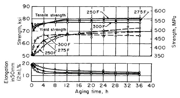
Figure 2: Aging curves devised for 7055 sheet when held at 120 to 150 $^{\circ}$ C (250 to 300 $^{\circ}$ F) [4].
