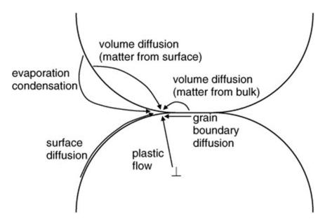
Figure 7: Mass transport mechanisms operative during solid state sintering.
