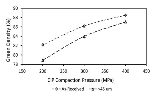
Figure 15: Compressibility curves for the two cuts of PA7055 powder studied.
