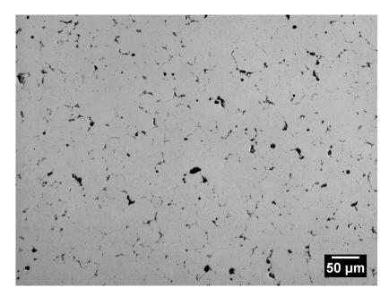
Figure 20: Microstructure of As-Received PA7055 powder admixed with 0.5% tin and sintered at 580°C.
