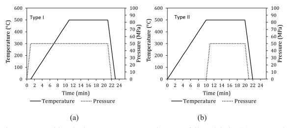
Figure 30: Transitions in the SPS temperature and pressure followed during (a) Type I and (b) Type II processing.
