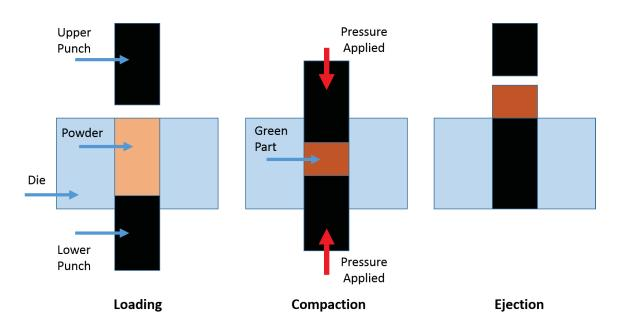
Figure 4: Schematic illustration of the UDC process.
