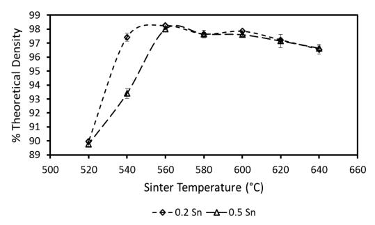
Figure 19: Effects of admixed tin additions on the sintering behaviour of As-Received PA7055 powder.
