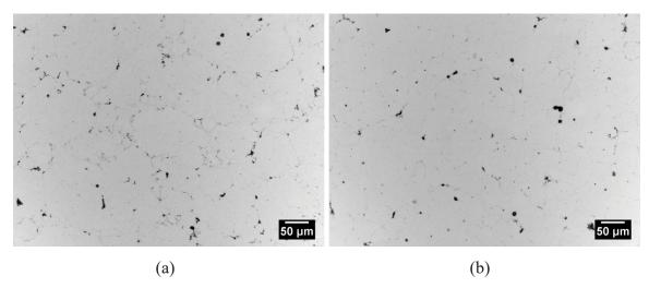
Figure 21: Microstructures observed in industrially sintered specimens of (a) As-Received and (b)  $>45 \mu m$  PA7055 powder. Both materials originally CIPed at 400 MPa and contained 0.2% tin.
