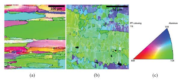
Figure 26: Maps illustrating the crystallographic orientations of  $\alpha$ -aluminum grains found within (a) CIP-Sinter-Forged-PA7055-T76 and (b) wrought 7055-T76 coupled with (c) the corresponding inverse pole figure. White lines indicate LAGBs whereas black lines indicate HAGBs.
