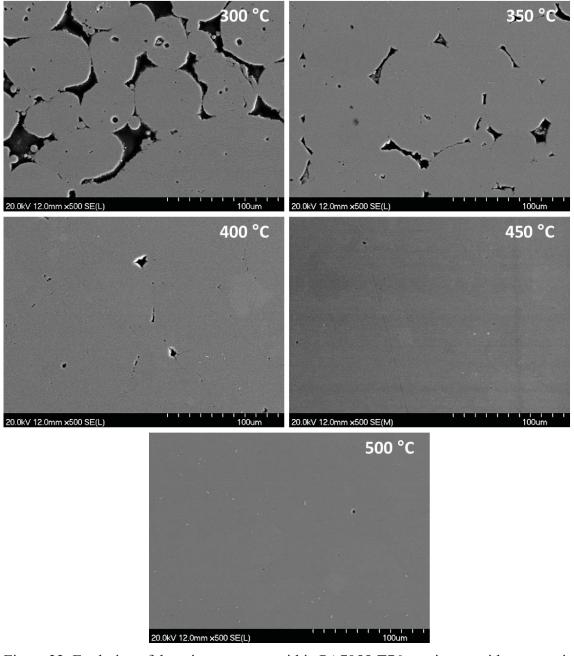
Figure 32: Evolution of the microstructure within PA7055-T76 specimens with progressive increases in SPS temperature. All specimens held at temperature for 120s (Type I). Porosity is black.
