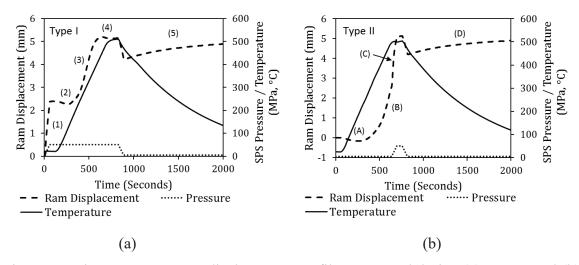
Figure 37: Figure 10: SPS ram displacement profiles measured during (a) Type I and (b) Type II processing sequences. Samples sintered at 500°C with a 120s hold time.
