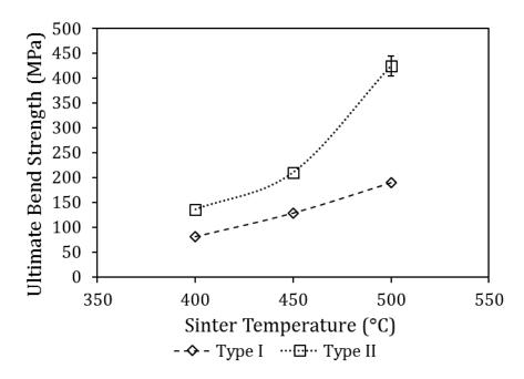
Figure 34: Effect of SPS temperature and loading mode on the UBS of PA7055-T76 specimens. All products held at temperature for 120s.
