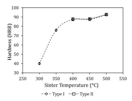
Figure 33: Effect of SPS temperature on the hardness of PA7055 specimens following T76 heat treatment. All specimens held at temperature for 120s.
