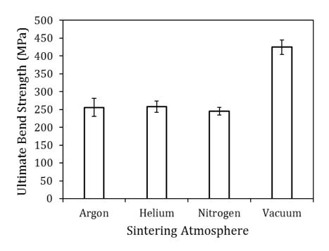
Figure 38: Effect of sintering atmosphere on the ultimate bend strength of PA7055 specimens consolidated at 500°C (Type II; 120s hold time).
