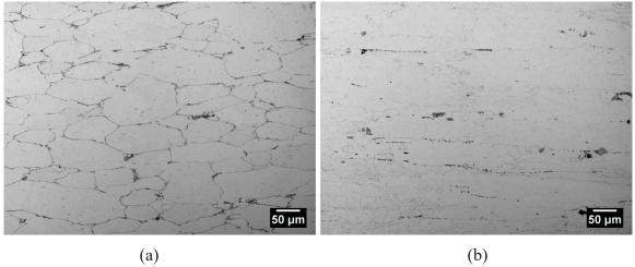
Figure 25: Comparison of the microstructures observed via optical microscopy in (a) CIP-Sinter-Forged-PA7055-T76 and (b) wrought 7055-T76 after etching with Keller's reagent.
