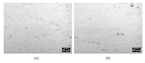
Figure 40: Microstructure of 7055 specimens (a) SPS-Forged-PA7055-T76 and (b) Wrought 7055-T76.
