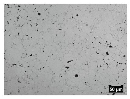
Figure 17: Microstructure of PA7055 (As-Received) after sintering at 580°C.
