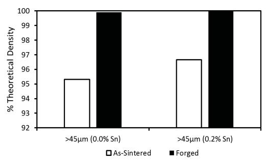
Figure 23: Effects of forging on the density of industrially sintered samples prepared with >45 μm PA7055 powder. All samples pre-heated at 470°C prior to forging.
