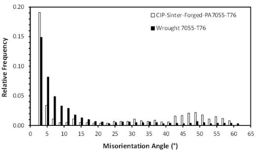
Figure 27: Comparison of the statistical distributions in grain misorientation angles for CIP-Sinter-Forged-PA7055-T76 and wrought 7055-T76.
