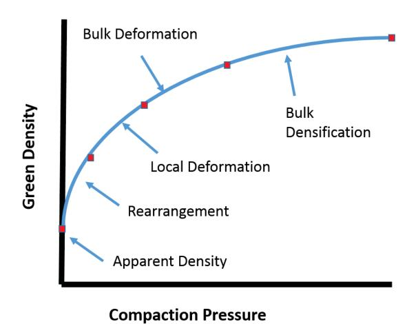
Figure 6: General description of the transition in green density as a function of applied compaction pressure.
