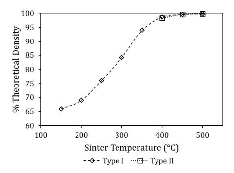
Figure 31: Effect of SPS temperature on the densification of PA7055 powder. All specimens held at temperature for 120s.
