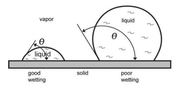
Figure 8: Comparison of good and poor wetting behavior for a liquid [29].
