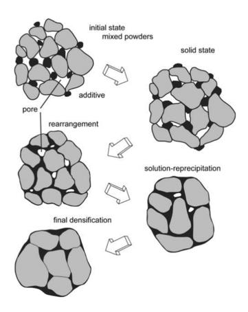
Figure 9: A schematic of the microstructure changes during LPS [29].
