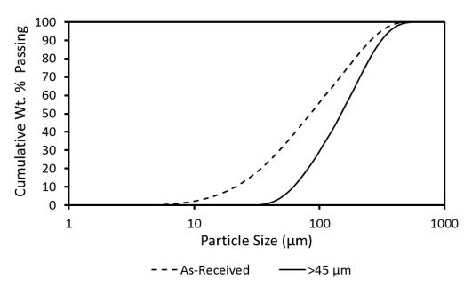
Figure 14: Particle size distributions for the two cuts of PA7055 powder studied.
