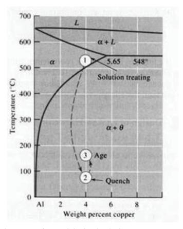
Figure 1: A typical sequence for precipitation hardening.
