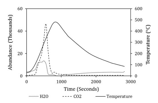
Figure 36: Off-gassing of H<sub>2</sub>O and CO<sub>2</sub> from PA7055 powder as a function of temperature.
