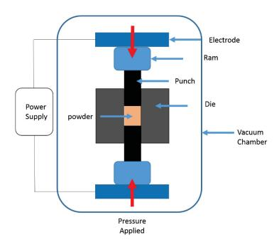
Figure 11: Schematic of a typical SPS system.
