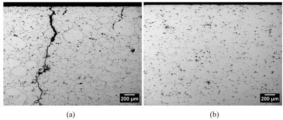
Figure 22: Comparison of the as-forged microstructures observed within samples prepared from (a) As-Received and (b)  $>45\mu m$  powders. Both materials contained 0.2 wt. % tin and were forged at  $470^{\circ}$ C.
