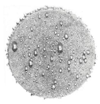
Figure 10: Image of a sample wherein the liquid phase was non-wetting and was thereby forced to the compact surface where it solidified as small spheres [29].
