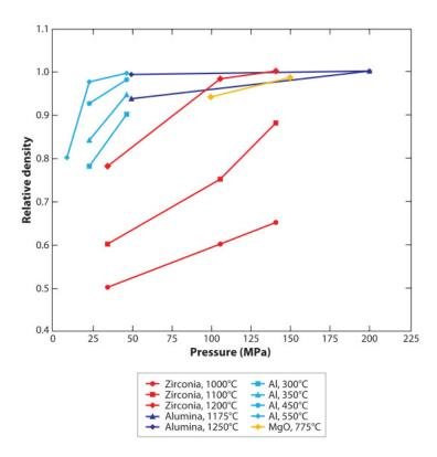
Figure 12: Densification response of various materials when processed through SPS [52].
