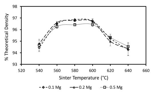
Figure 18: Effects of admixed magnesium on the sintering behaviour of As-Received PA7055 powder.
