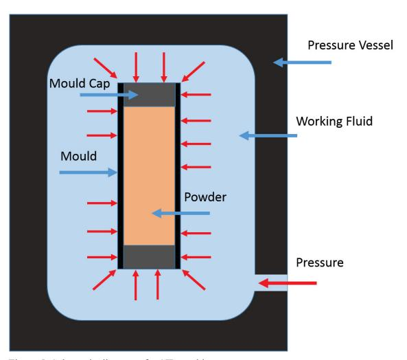
Figure 5: Schematic diagram of a CIP machine.
