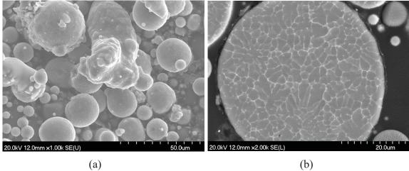
Figure 29: Images illustrating the typical (a) morphology and (b) internal microstructure of PA7055 powder.
